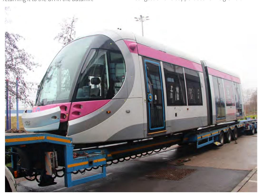
Further tests will then be carried out at the Metro depot before work begins there on fitting out the rest of the 21-tram fleet. The Midland Metro will be the first commercial tram system in the UK to have catenaryfree running, allowing the trams to operate over short distances without the need for overhead cables and equipment.
