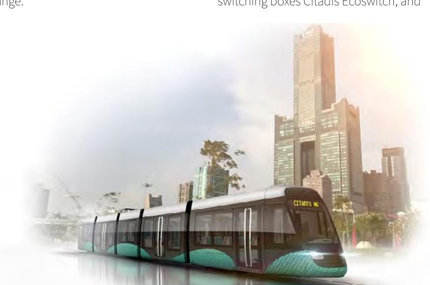
Alstom will provide Citadis X05 which is equipped with the latest technologies including permanent magnet motors to reduce energy consumption. Alstom will also equip the trams with its Citadis Ecopack, an on-board energy storage solution located on the roof which enables the tram to run without a catenary from a station to another. Citadis Ecopack enables the tram to be fully charged through the catenary when stopped at stations in 20 seconds.
