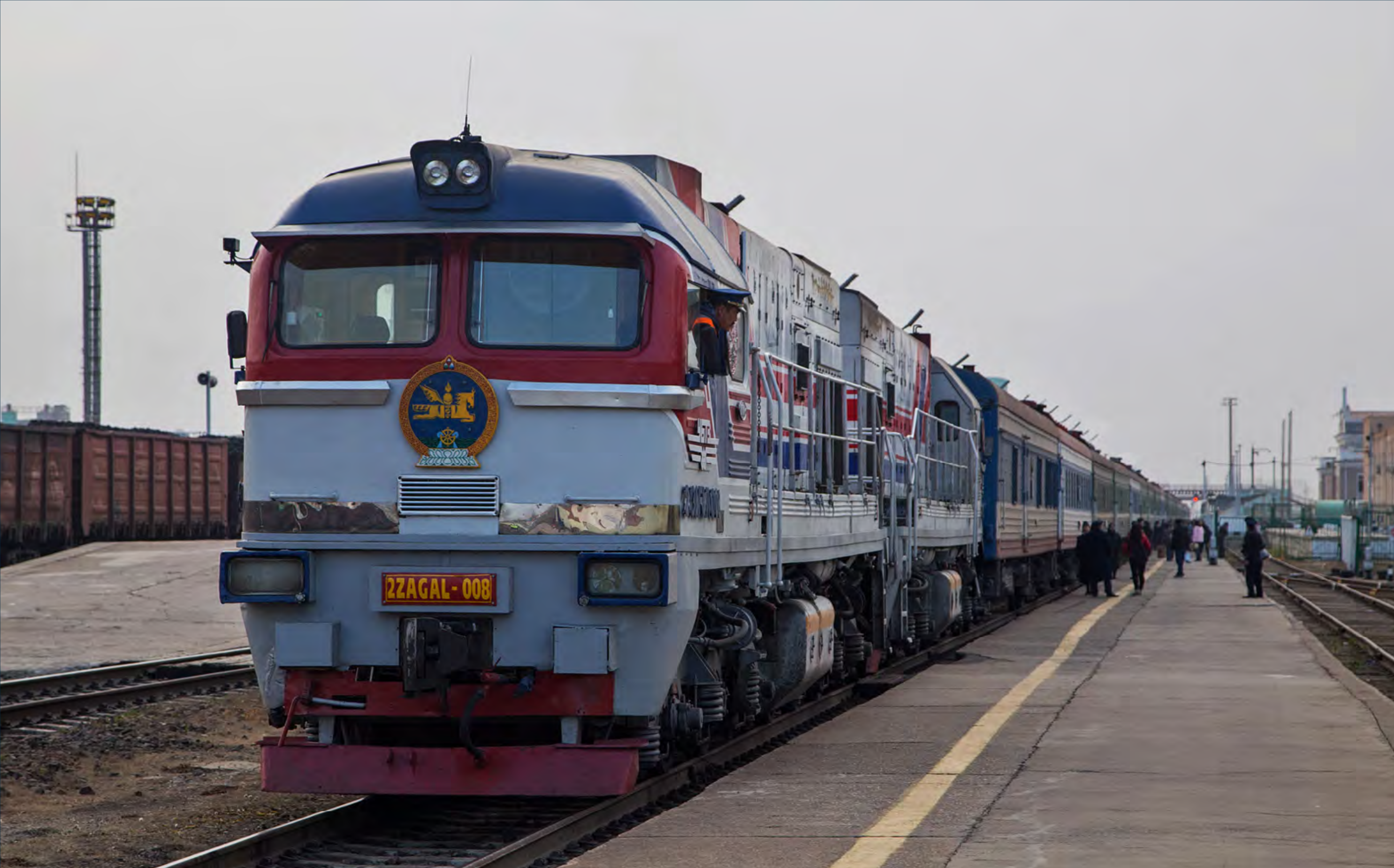
▶ On October 21st, No. 2ZAGAL 008 A+B stands at Ulaan Baatar with train No. 276 to Zamyn Uud. These locos are former 2M62s rebuilt with GE engines. Mark Torkington
