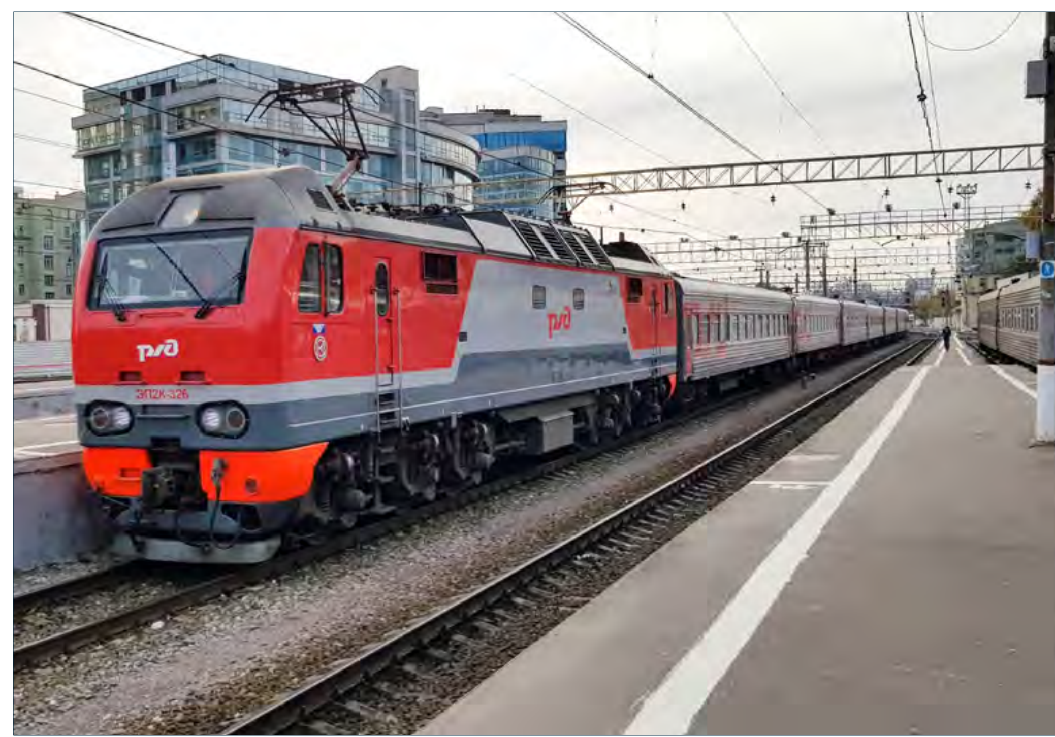
▶ The EP2K electric locomotive was designed to haul passenger trains on 1520mm gauge railways powered by 3kV DC, here No. EP2K-326 arrives at Moscow Paveletski on October 13th. Mark Enderby
