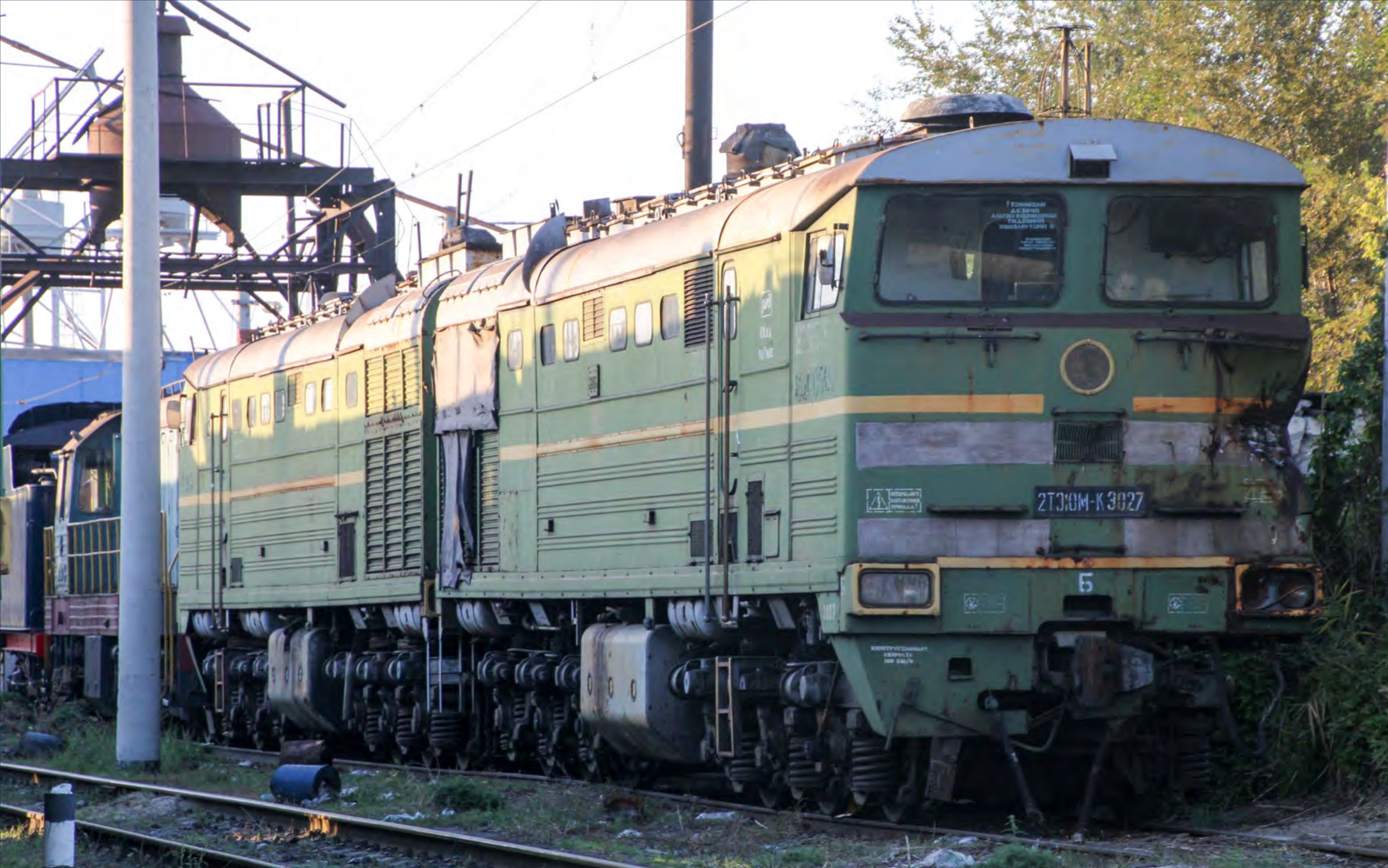
▶ Soviet-Ukrainian diesel-electric locomotive No. 2TE10M-K3027 with collision damage, stabled on Tikhoretsk depot on October 9th. Mark Enderby
