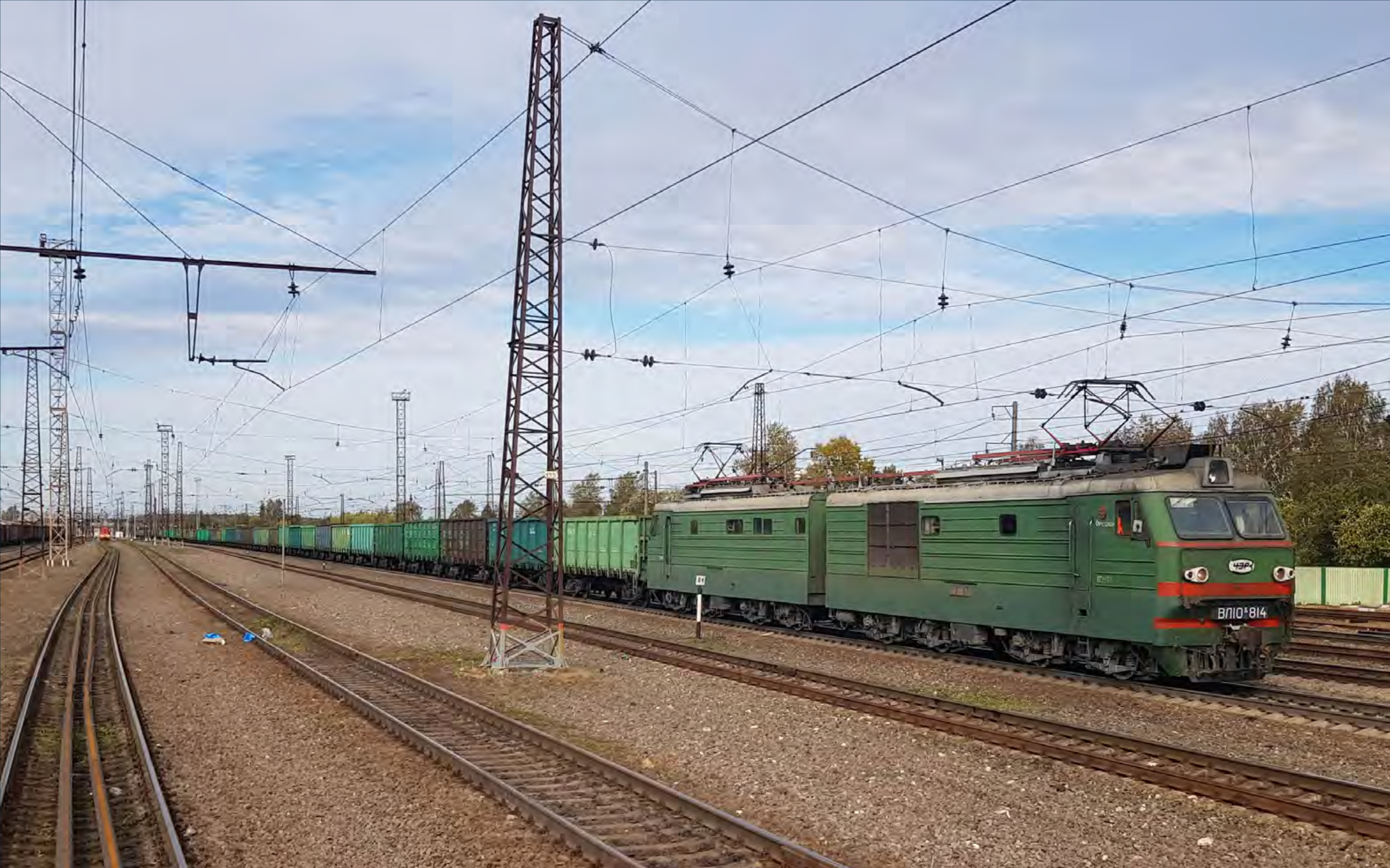
VL10 electric two-unit mainline DC freight locomotive No. VL10-814 passes Voskresensk on October 1st. Mark Enderby
