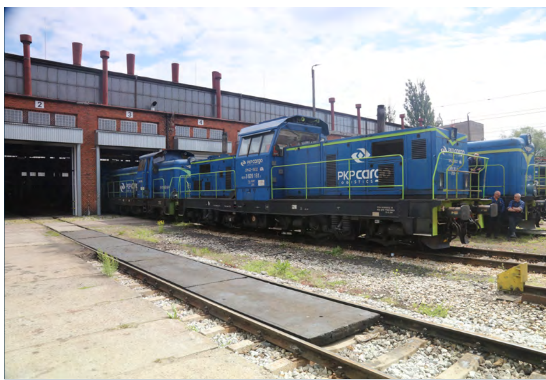
▶ On June 2nd, Nos. SM42-922 and SM42-1602 gingerly make their way into Poznan Franowo depot for servicing. Note that the nearer loco has had the bonnet tops reduced in height to give better visibility from the cab. Jeff Nicholls
