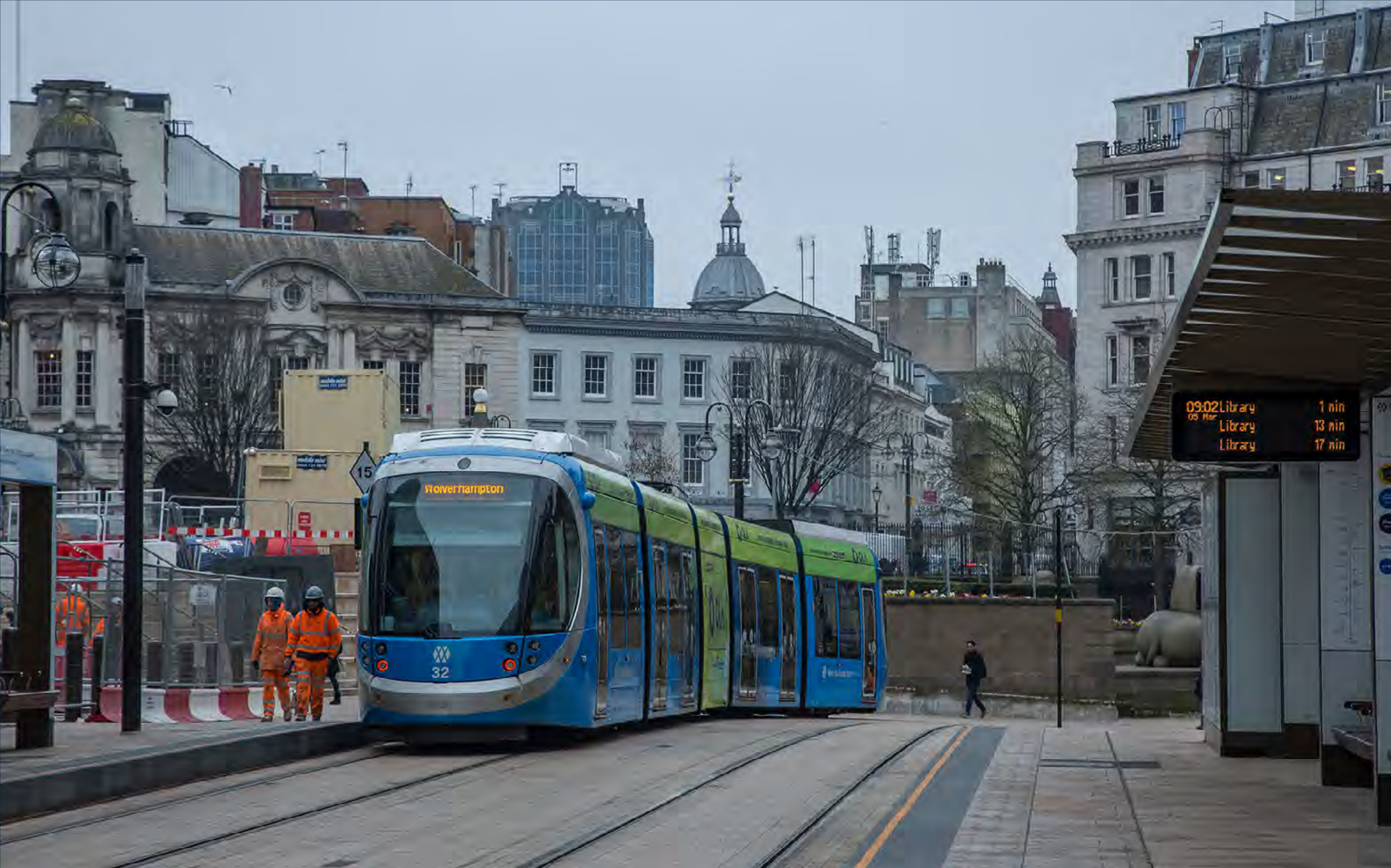
▶ Tram No. 32 departs Centenary Square stop running on battery power, heading towards the city centre. Richard Hargreaves
