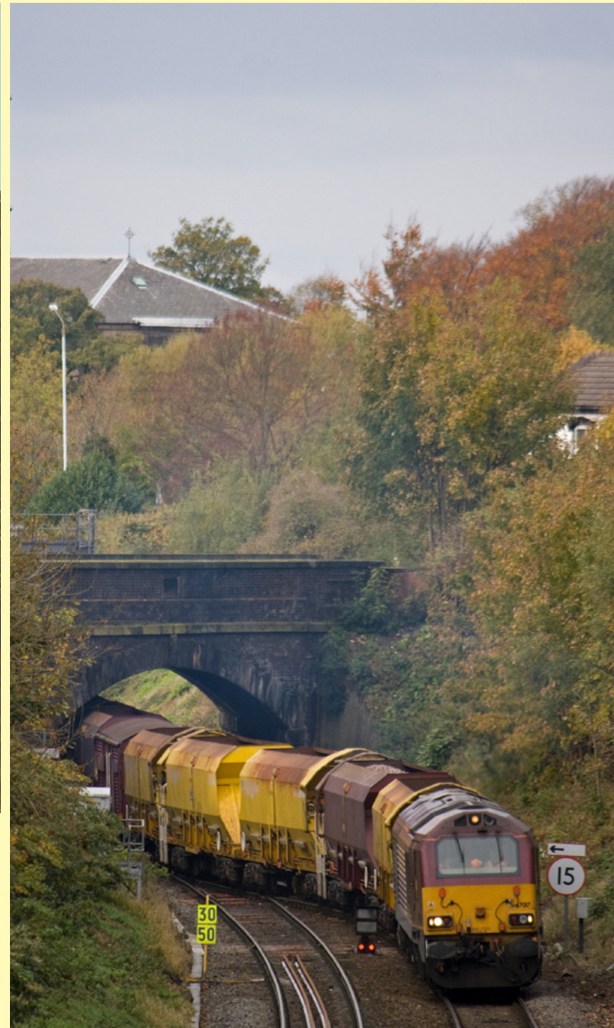
Right: Class 67 017 with 66 105 on the rear, works the 6Z60 Bescot - Wellington Regent Street on the 29th October. The train was dropping ballast on the new Telford Freight Terminal branch as far as Hadley. The terminal is due to open Spring 2009. Carl Grocott
