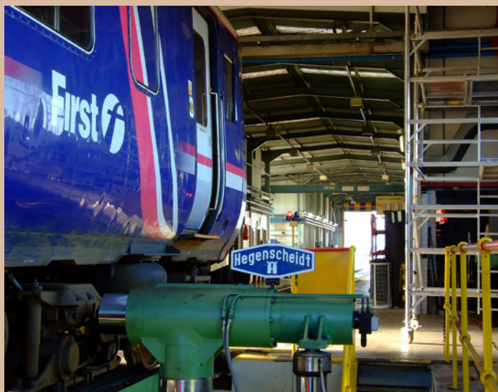
Above: Another shot of Class 156 476 (52476 end) seen inside the wheel lathe shed at Shields having its wheels turned.
