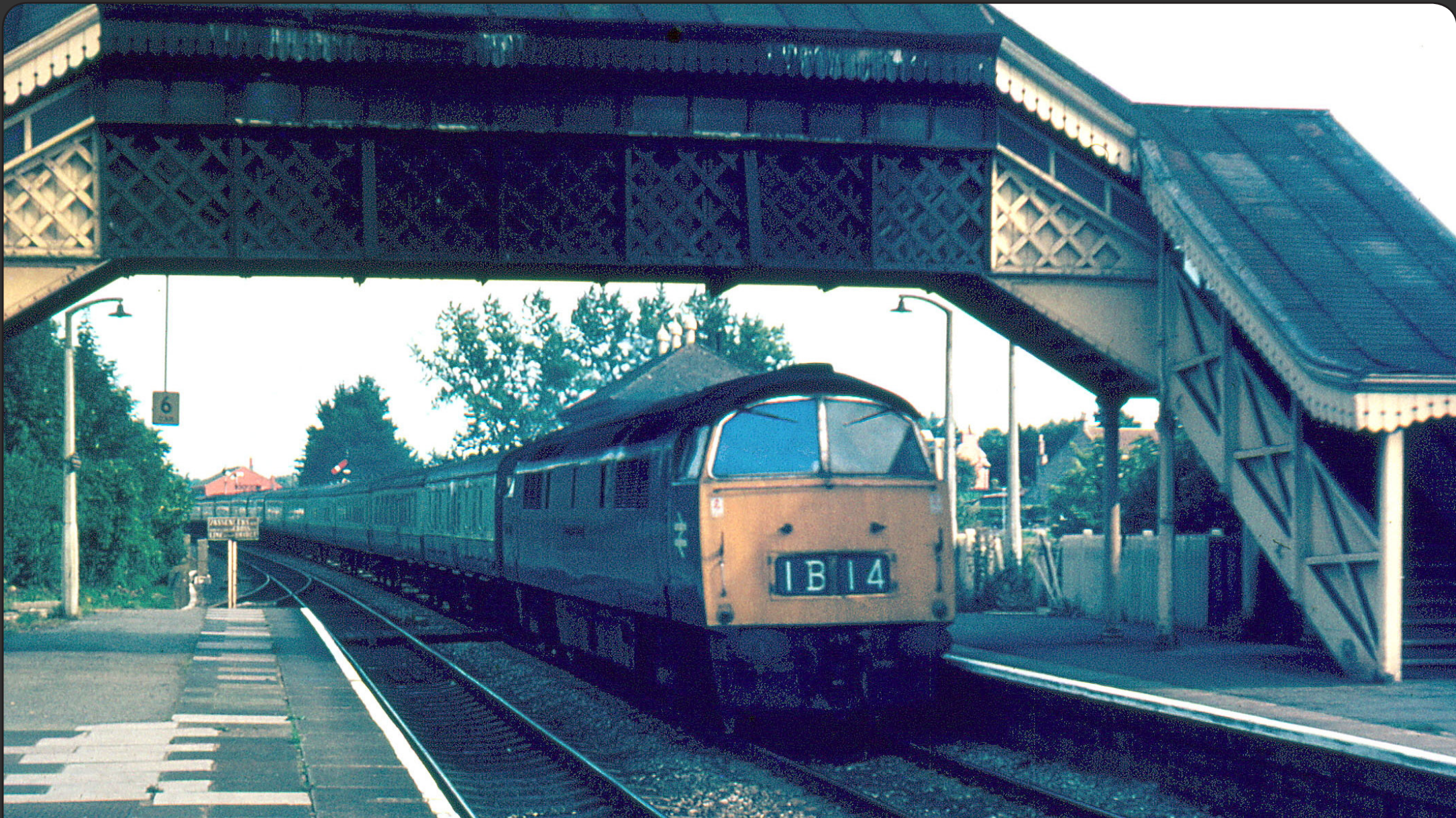
For many years, the Class 52s were predominant working both passenger and freight trains on the Western Region. They were introduced in 1961 and were built both at Swindon and Crewe Workshops. They became very popular with enthusiasts as they consisted of two Maybach V-type engines, which certainly made a noise at speed! Here D1059 Western Empire is seen on September 1st 1969 working the 14.45 London Paddington - Bristol Temple Meads passing Keynsham, prior to the demolition of the GWR footbridge. David Mead
