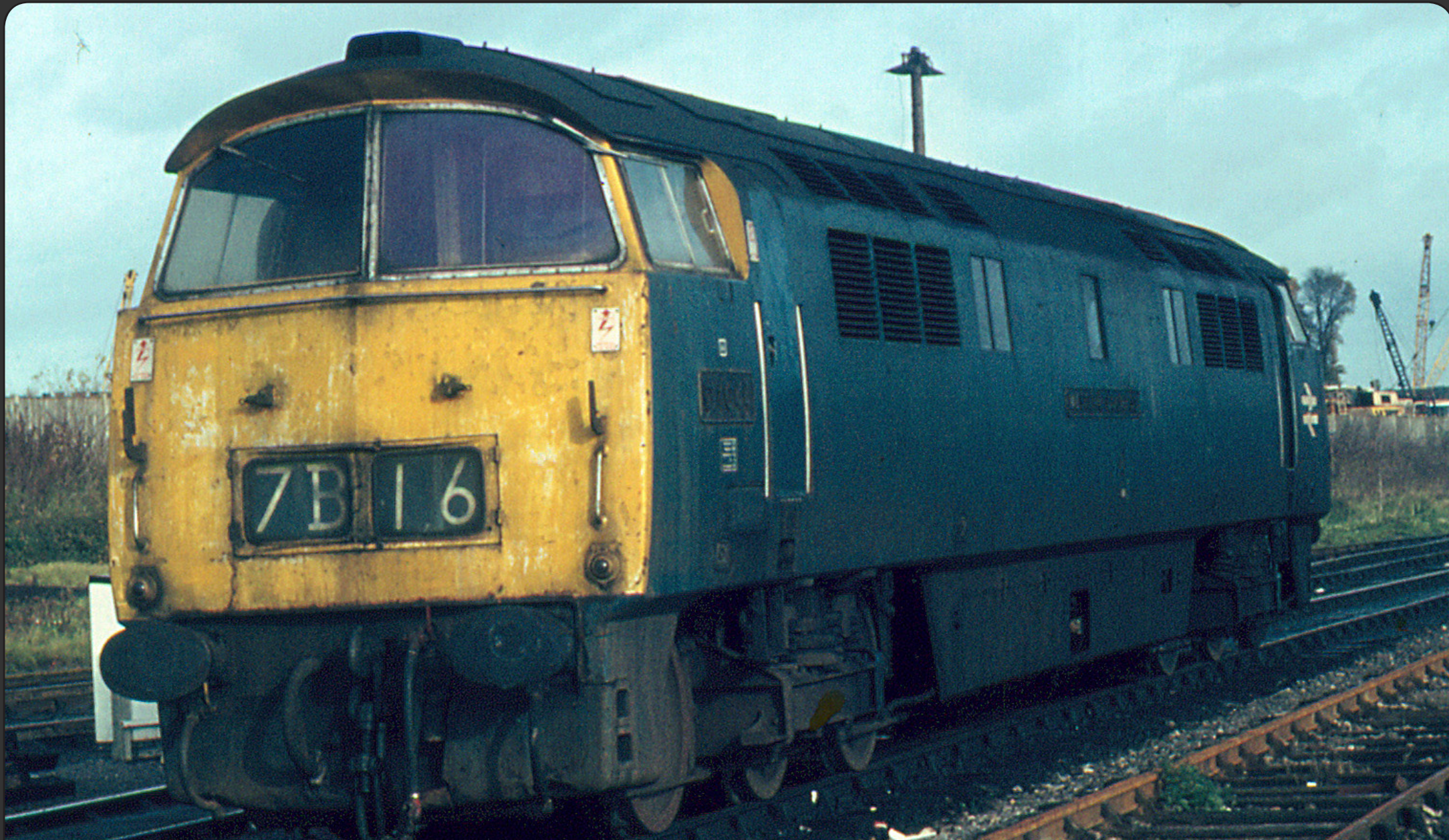
On a visit to Westbury on November 10th 1974, D1044 Western Duchess stands on the depot yard waiting its next duty. By this time, the locomotives were known as Class 52s and the "D" had been painted out on most of the number places. During the 1970's, the Class 52's were the main power for the Merehead and Whatley Quarries stone trains and the Maybach power certainly was taken at full strength working the gradient from Westbury towards Warminster. David Mead
