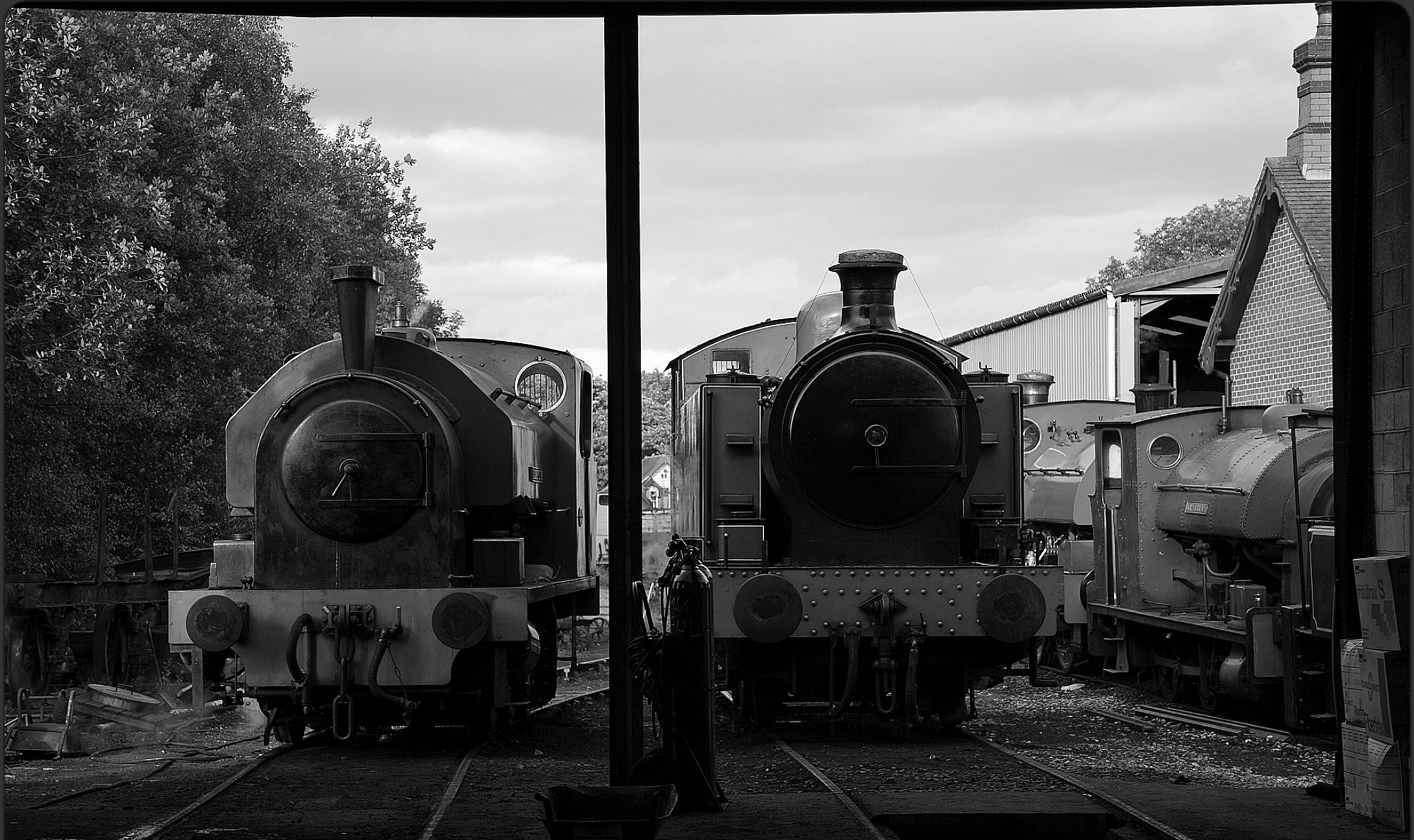
At Foxfield's Caverswall Road depot are No. 3059 "FLORENCE" a Giesel ejector loco with characteristic tapered chimney which was built in 1954 and No. 1684 "MEAFORD No .2" a Newcastle upon Tyne outside cylindered loco which was built in 1951. Richard Hargreaves
