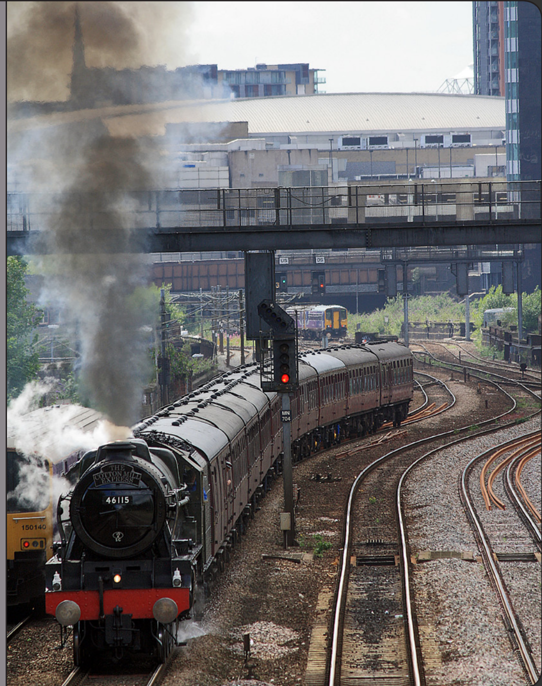
Right: After hammering the final nail into the coffin of the Cotton Mill Express, LMS Royal Scot 7P 4-6-0 No. 46115 "Scots Guardsman" slowly ascends Miles Platting bank on July 17th having been declared a failure with a broken middle cylinder at Manchester Victoria. The engine had just completed 1 out of 2 loops of the route via Huddersfield and Copy Pit, and as it's third time unlucky (again) this sight may never be repeated. CJ Sutcliffe
