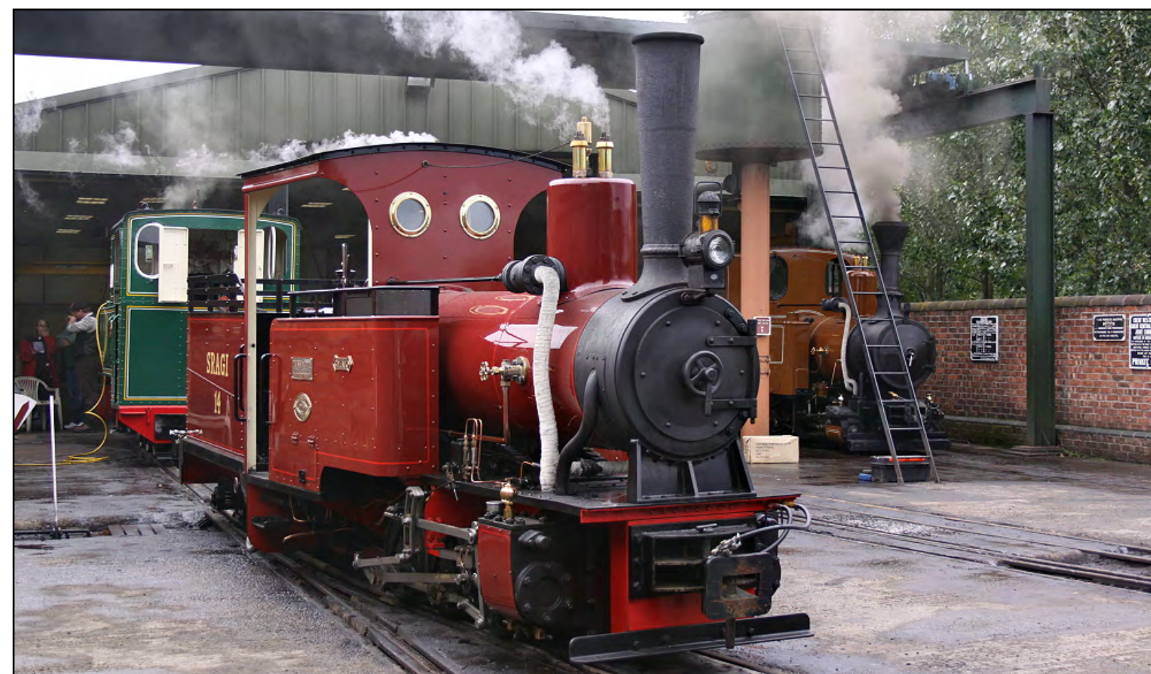
Above: SACCHARINE. An 0-4-2T built by Fowler in 1914 to works No. 13355. As the name tends to suggest, the locomotive was originally built for use in a sugar plantation in South Africa. Pete Cheshire Below: SRAGI No. 14,"MAX" built by Orenstein & Koppel to works number 10750 in Berlin. Sragi is the largest sugar mill in Central Java, Indonesia, with an extensive 600mm guage system, operating steam locomotives from 9 different European manufacturers. Pete Cheshire
