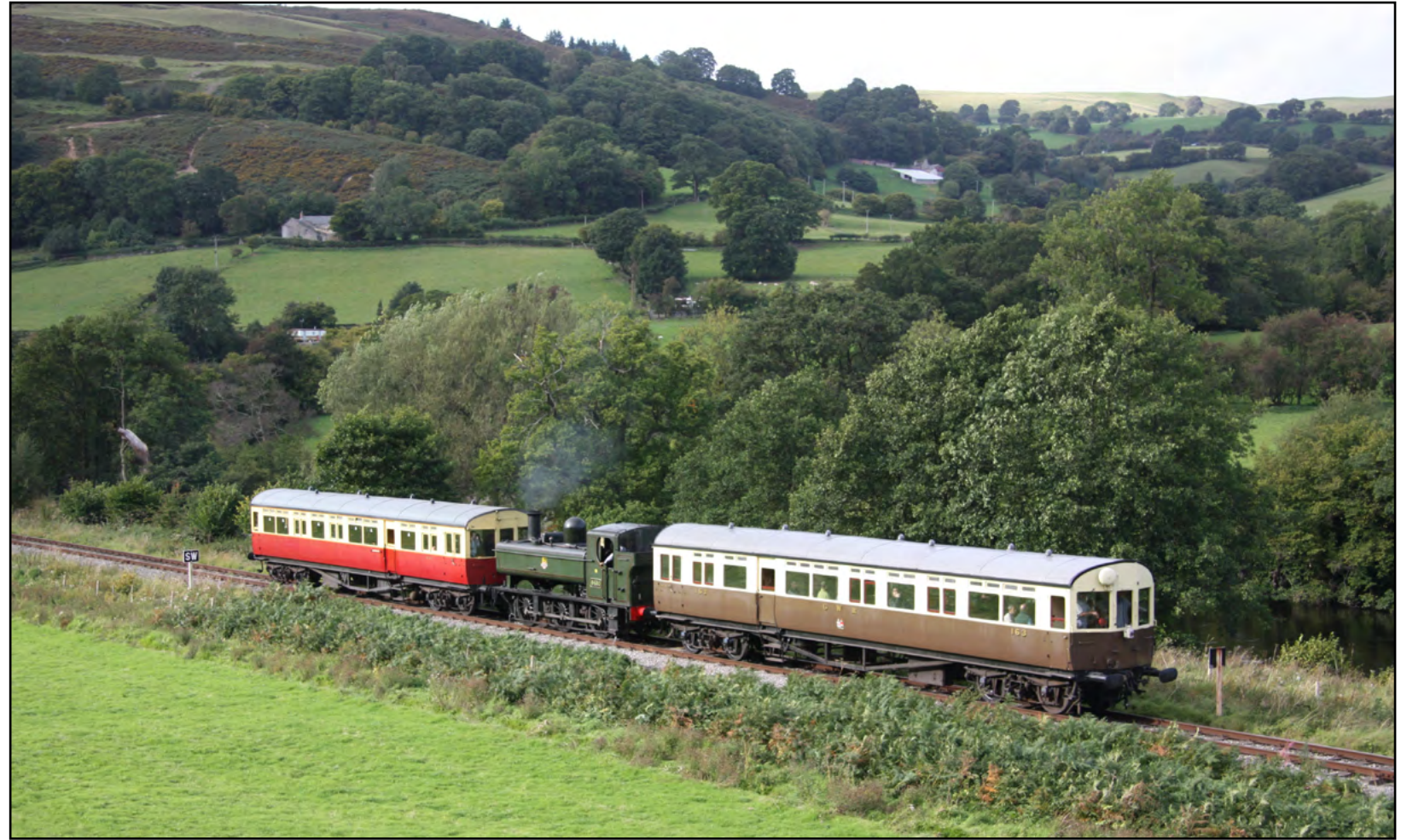
Below: GWR No. 6430 is a push-pull fitted 0-6-0 pannier tank, seen here working the auto train. Phil Martin Bottom: Great Western Railway No. 4953 "Pitchford Hall" works the 16.45 ex Llangollen on September 12th. Phil Martin
