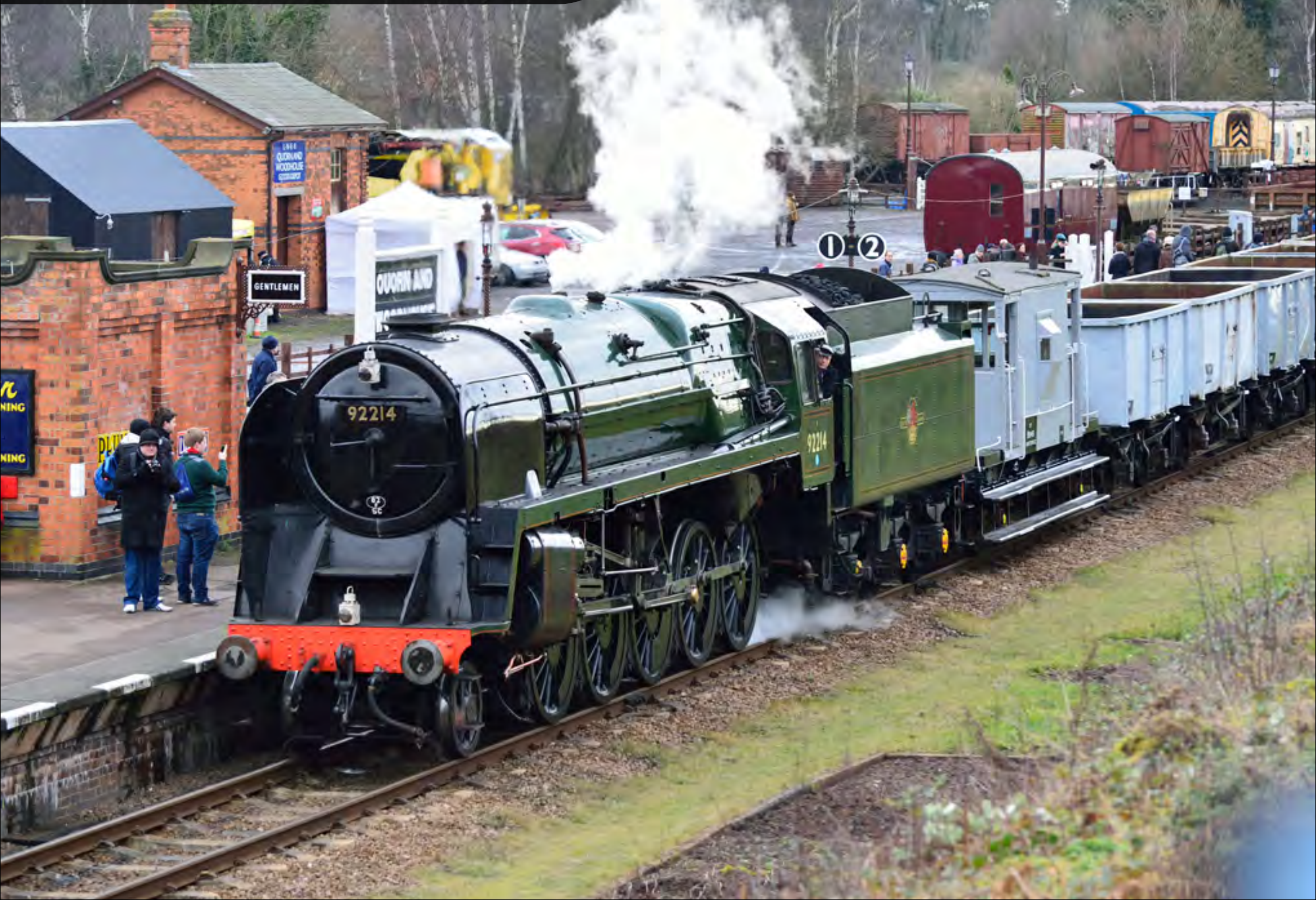
BR Standard 9F 2-10-0 heavy freight locomotive No. 92214 makes light work of hauling a rake of empty mineral wagons through Quorn and Woodhouse station, heading for Loughborough. Class47
