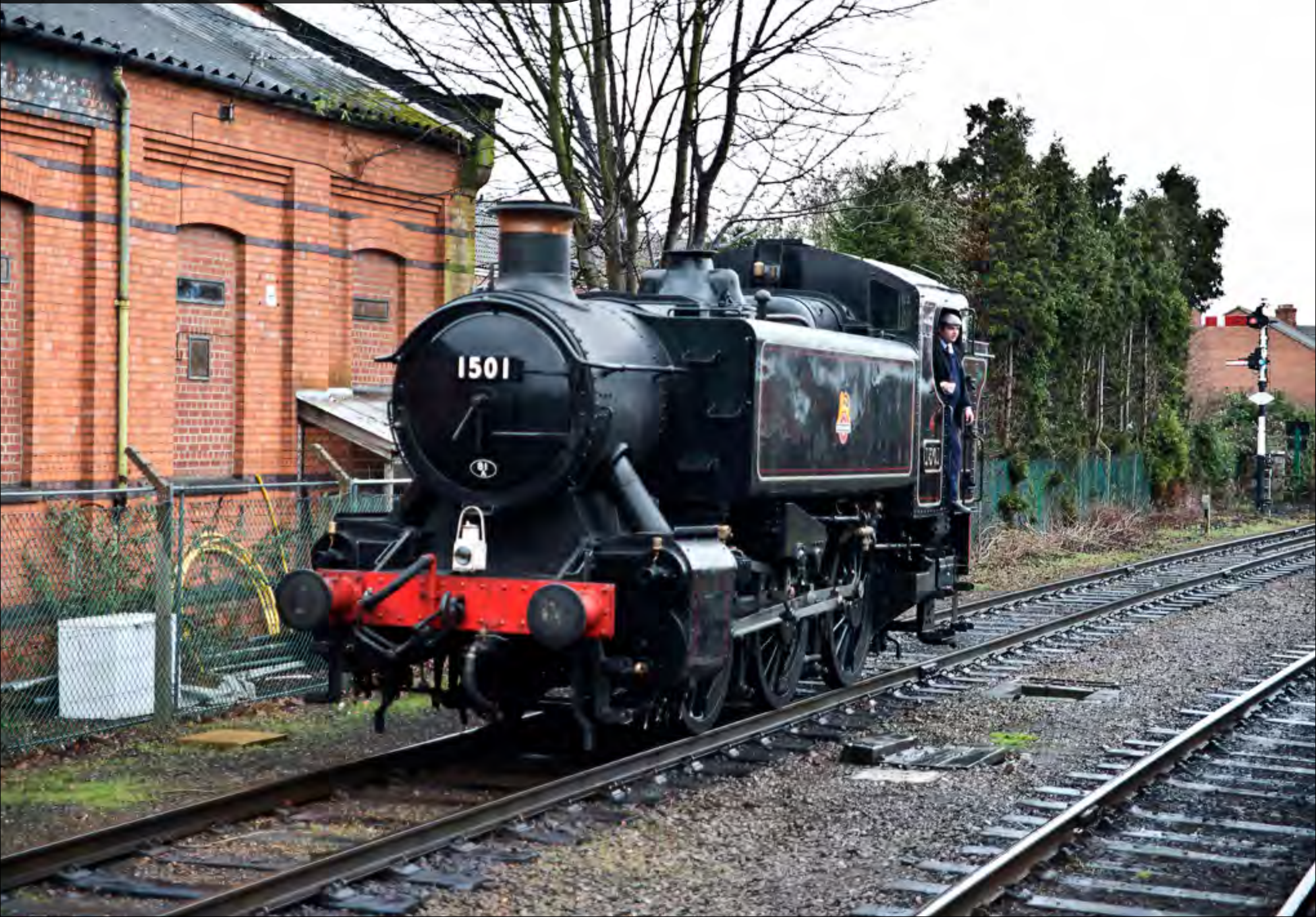
Great Western Railway (GWR) 1500 Class 0-6-0 pannier tank steam locomotive No. 1501 stands at Loughborough awaiting its next duty. Class47
