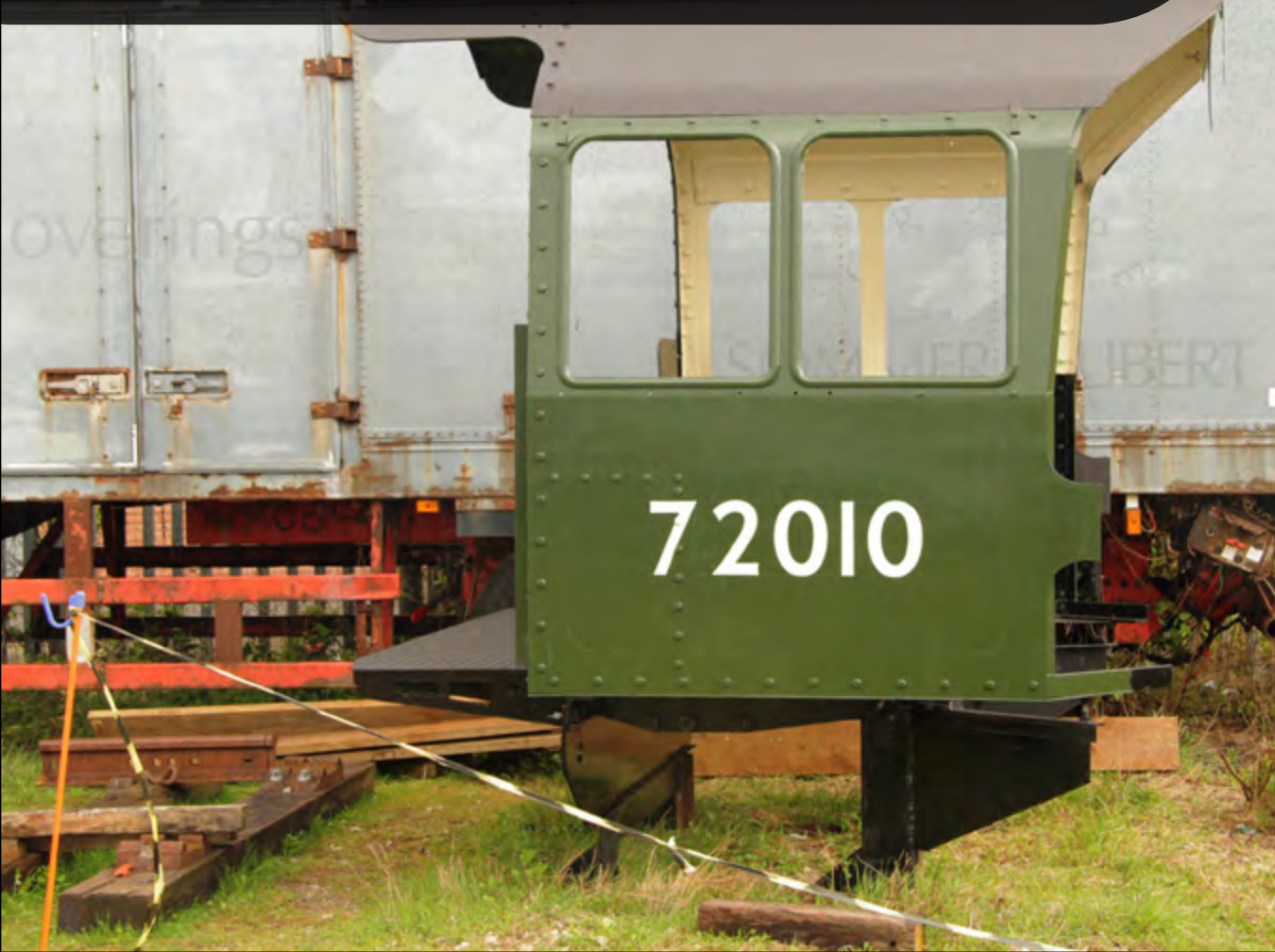
On May 7th, the cab of new build Clan Class loco is seen at Nemesis Rail, Burton upon Trent with the number having just been applied. Derek Elston
