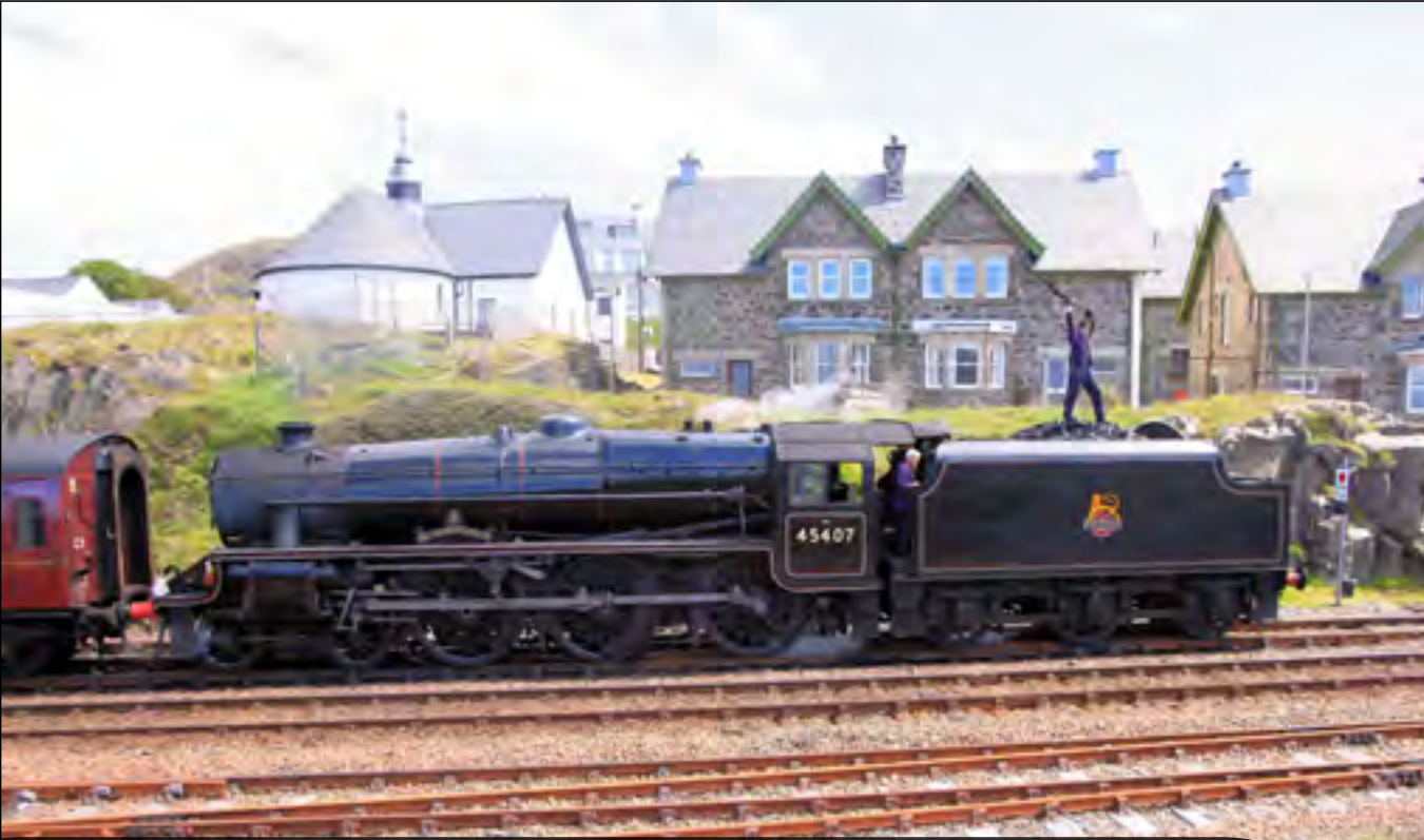
LMS Stanier Class 5 4-6-0 45407 'The Lancashire Fusilier' stands in Mallaig station on June 12th. The fireman is standing on the tender, shovel aloft, with the magnetic aerial attached in order that the driver can get a wireless link to speak to the signaller. Ah, the nostalgia of steam! Neil Pugh
