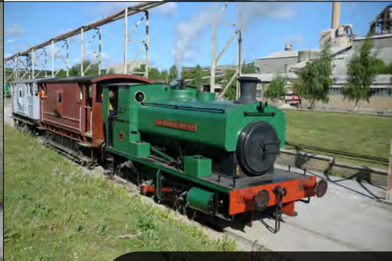
Rocks & Rail's Andrew Barclay 0-4-0ST 'Sir Thomas Royden' is pictured giving Brake Van rides at the open day. John Alsop
