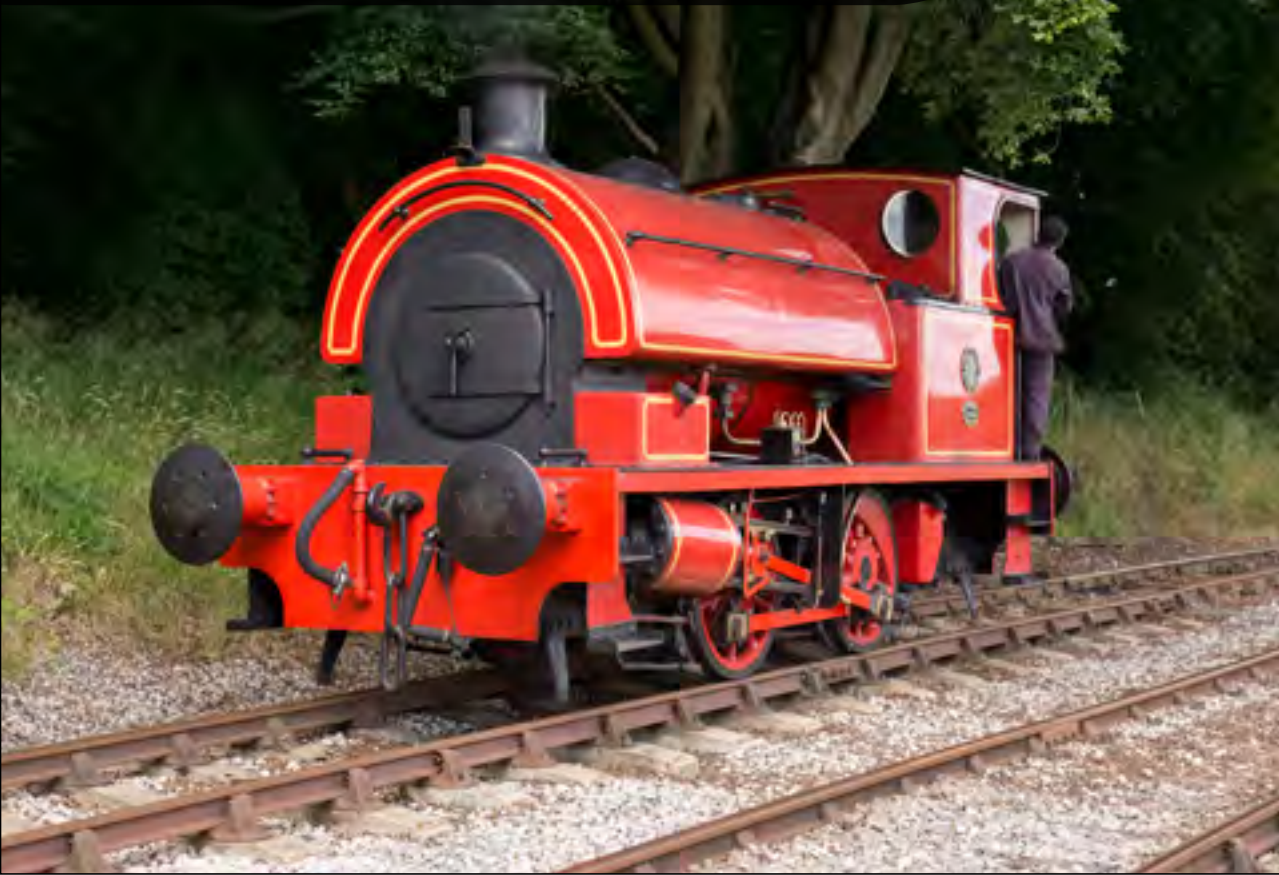
Bagnall 0-4-0 saddle tank built 1946, No. 2842 is seen at Dilhorne Park on July 19th. Brian Battersby
