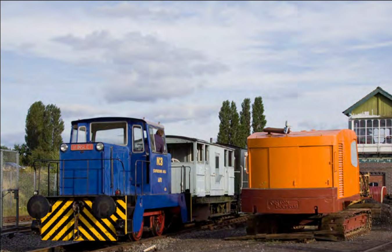
Hunslet 0-4-0 diesel hydraulic locomotive No. 6678 shunts some brake vans at Chasewater. Richard Hargreaves
