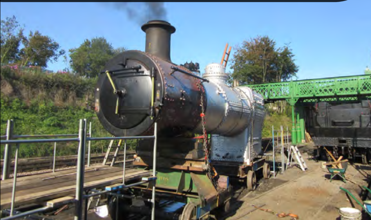
The boiler from Ivatt 2-6-2T No. 41312 boiler is seen on test at Ropley on September 28th. Ken Livermore
