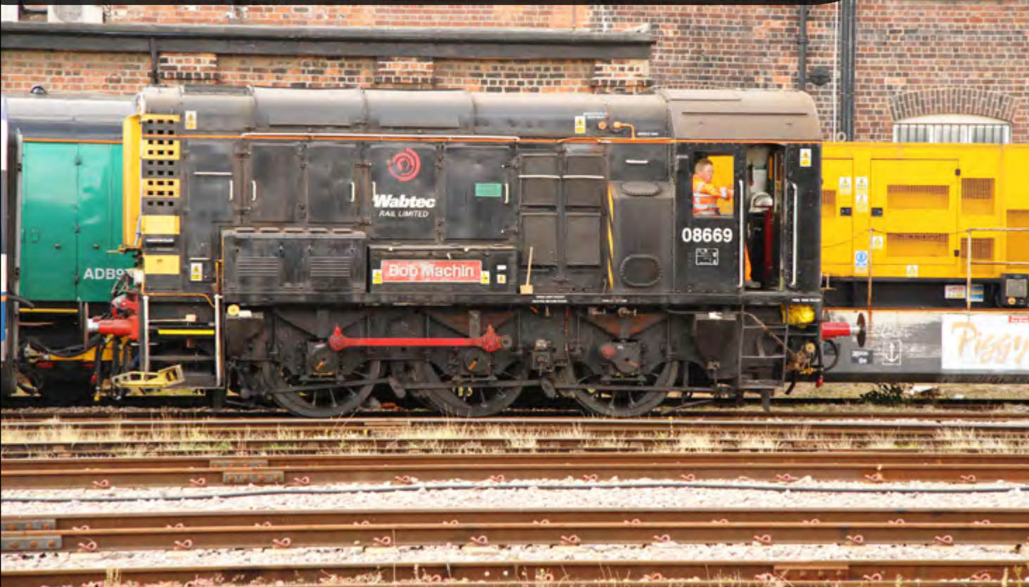
Wabtec shunter Class 08 669 'Bob Machin' is seen working alongside Doncaster works as an 0-4-2 with one set of wheels not connected. Derek Elston
