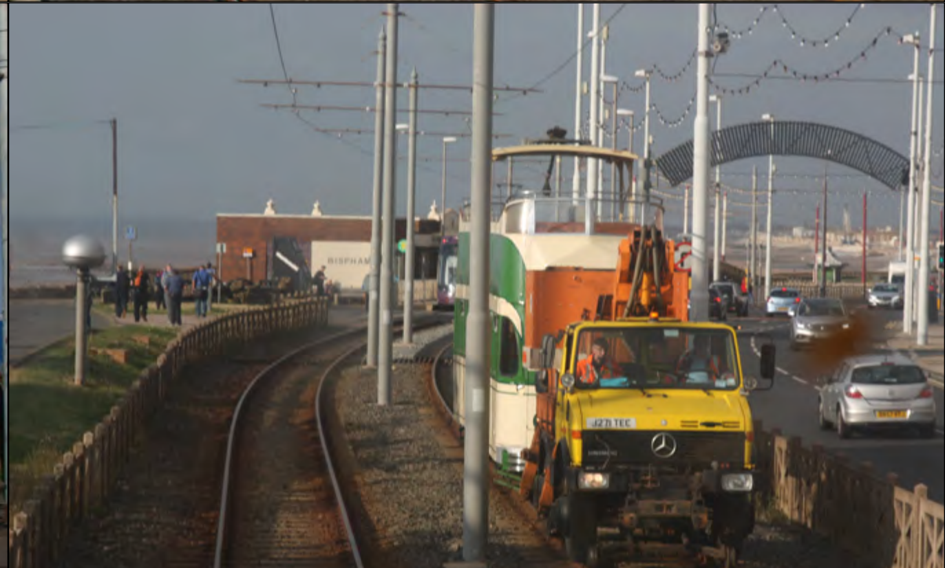
On September 26th, having had a mishap at Bispham whilst crossing over onto the wrong line ( it pulled the end off its pole), Balloon No. 706 had to be rescued by a road rail Unimog and is seen here being towed back to Rigby Road. Phil Martin
