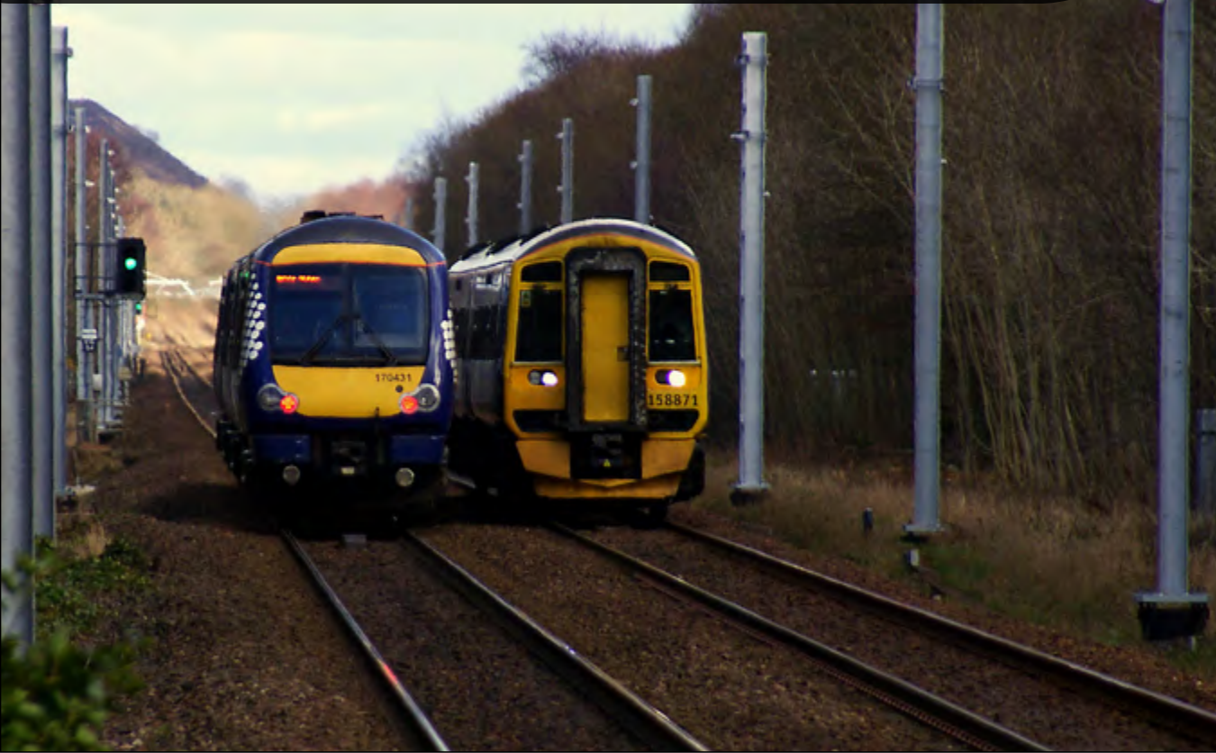
Class 158 871 passes 170 431 on the Edinburgh - Glasgow line at Lenzie, on February 24th. Clearly visible are the new masts in place for the overhead wires that are being fitted this year. Greig Gibson
