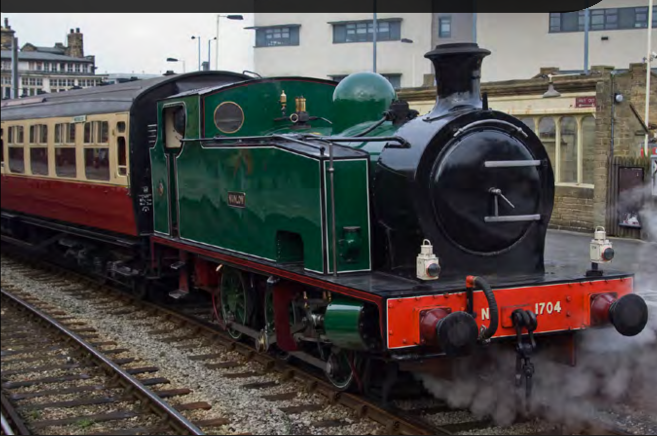
Hudswell Clarke & Co. Ltd. 0-6-0T side tank No. 1704 'Nunlow' is seen at Keighley on February 27th working a local train to Ingrow West. Richard Hargreaves
