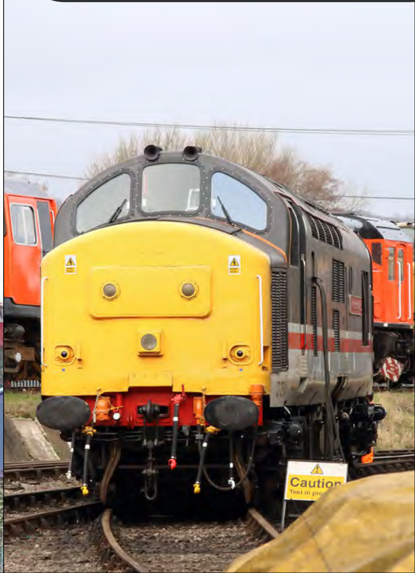
Former Spa Valley resident, Class 37 254 is seen undergoing load bank tests on February 20th. Class47
