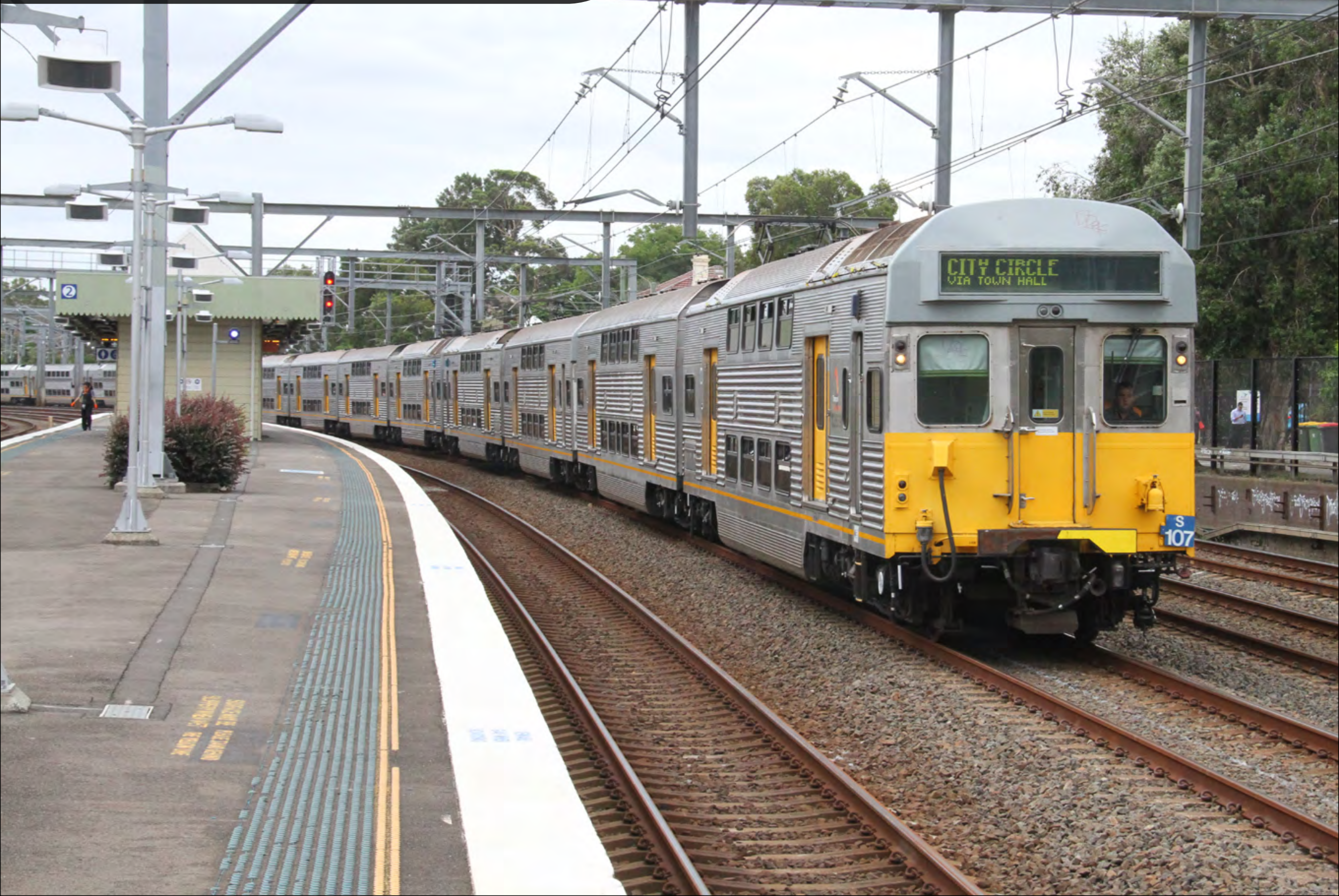
S Set power car No. 3889 leads a Sydney Trains suburban working through Summer Hill on December 2nd. The S sets are stainless steel, double deck construction and are not air conditioned. Anton Kendall
