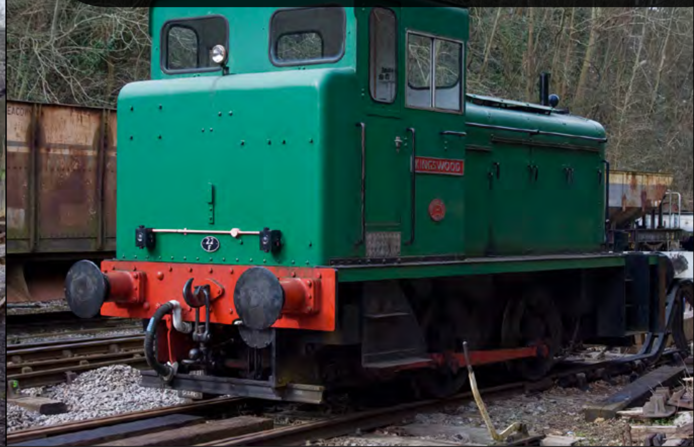
Former Central Electricity Generating Board (CEGB) Rogerstone power station shunter, Barclay 0-4-0DM 'Kingswood' awaits repairs. Richard Hargreaves
