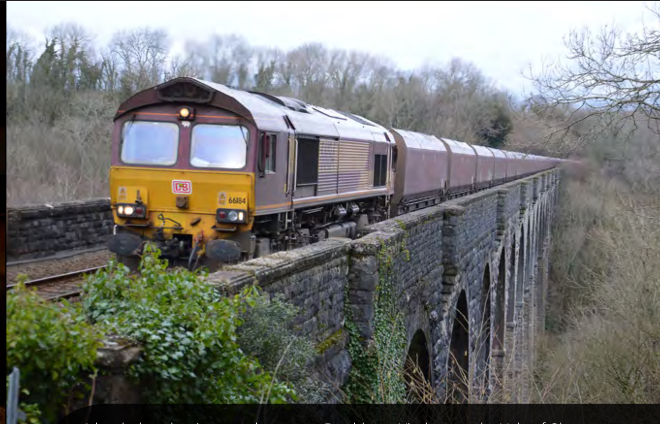
A loaded coal train struggles across Porthkerry Viaduct on the Vale of Glamorgan line (Barry to Bridgend) headed by Class 66 184 on an upward gradient of 1 in 87!! Ken Mumford
