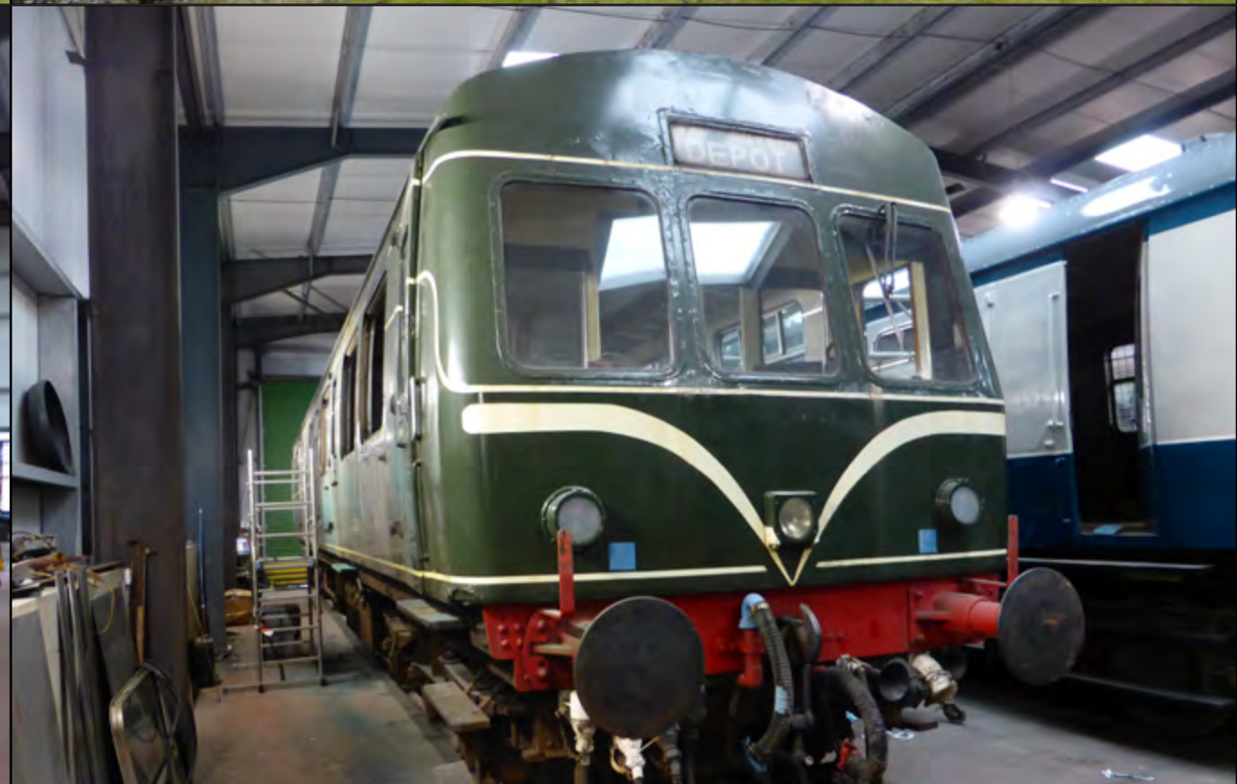
The Great Central Railway's Class 101 DMU No. E50321 is seen partially stripped at Rowsley, ready for a repaint. Andrew Wilson
