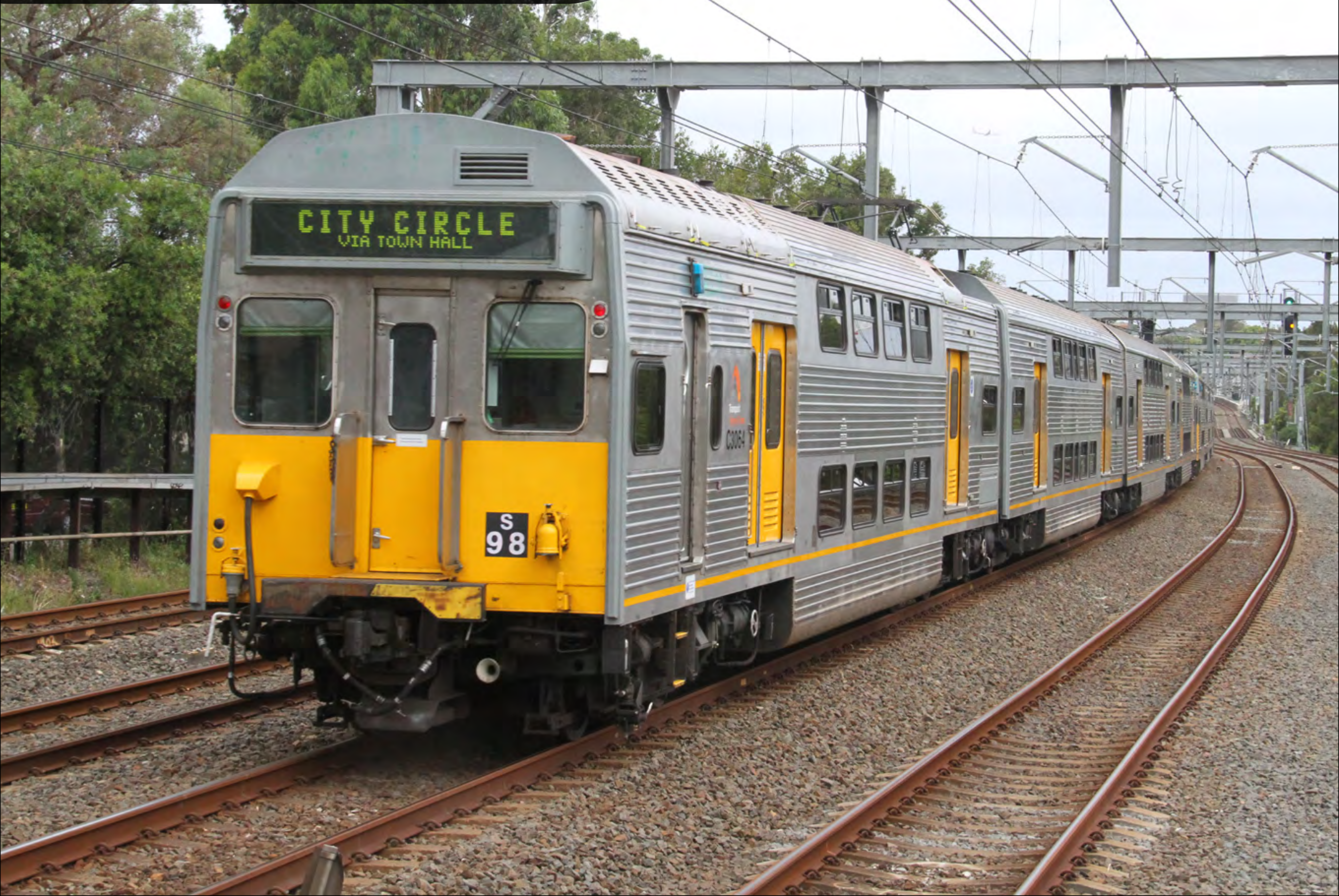
'S' Set power car No. 3064 leads a Sydney Trains suburban working through Summer Hill. The 'S' sets are stainless steel, double deck construction and are not air conditioned. Anton Kendall
