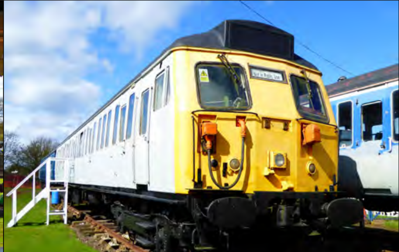
Former Great Eastern Class 308 136 BDTCoL No. 75881, believed to be the last vehicle of its class in existence. Nick Clemson
