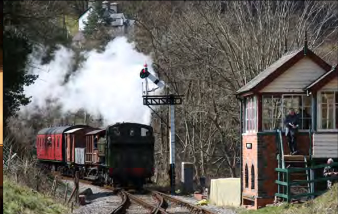
Great Western Railway 6400 Class 0-6-0 Pannier Tank No. 6430 approaches Glyndyfrdwy on April 10th with a mixed train working. Phil Martin
