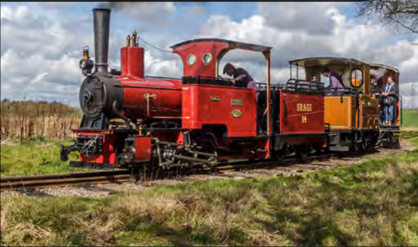
O&K 0-6-0WT (Works No. 10750 of 1923) No. 14 'Max' and Krauss 0-4-2T (Works No. 4045 of 1899) Sragi No. 1 are seen working round the balloon loop. Both locomotives were built in Germany for the Sragi Sugar Company in Java where they were still in use into the 21st century. Ken Abram
