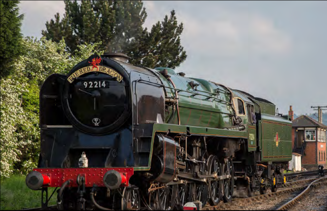
BR Standard Class 9F 2-10-0 No. 92214 heads out of the station at Toddington. Richard Hargreaves
