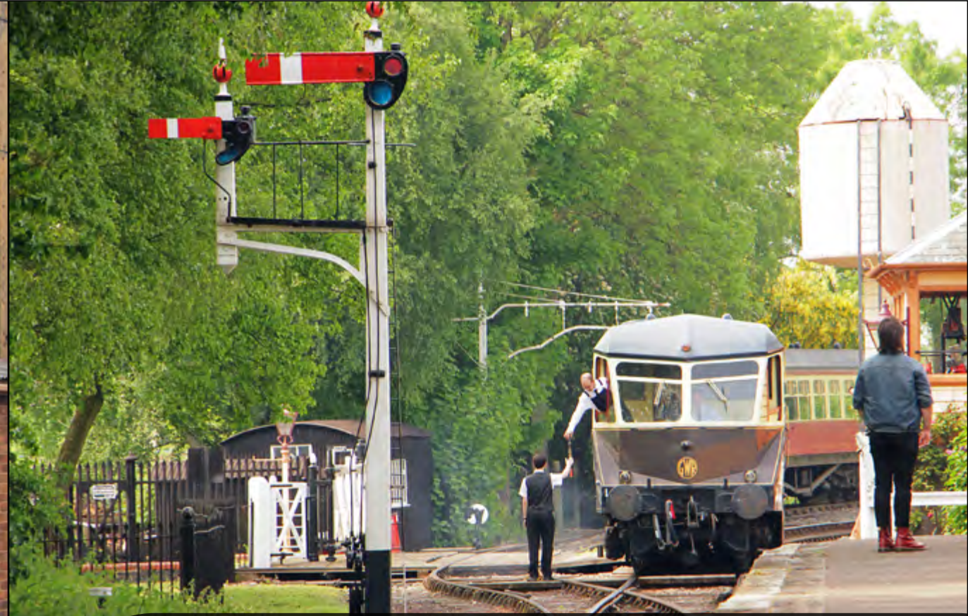
A branch line scene at Didcot on May 28th, as the second man on GWR Railcar No. 22 passes over the token to the signalman. Derek Elston
