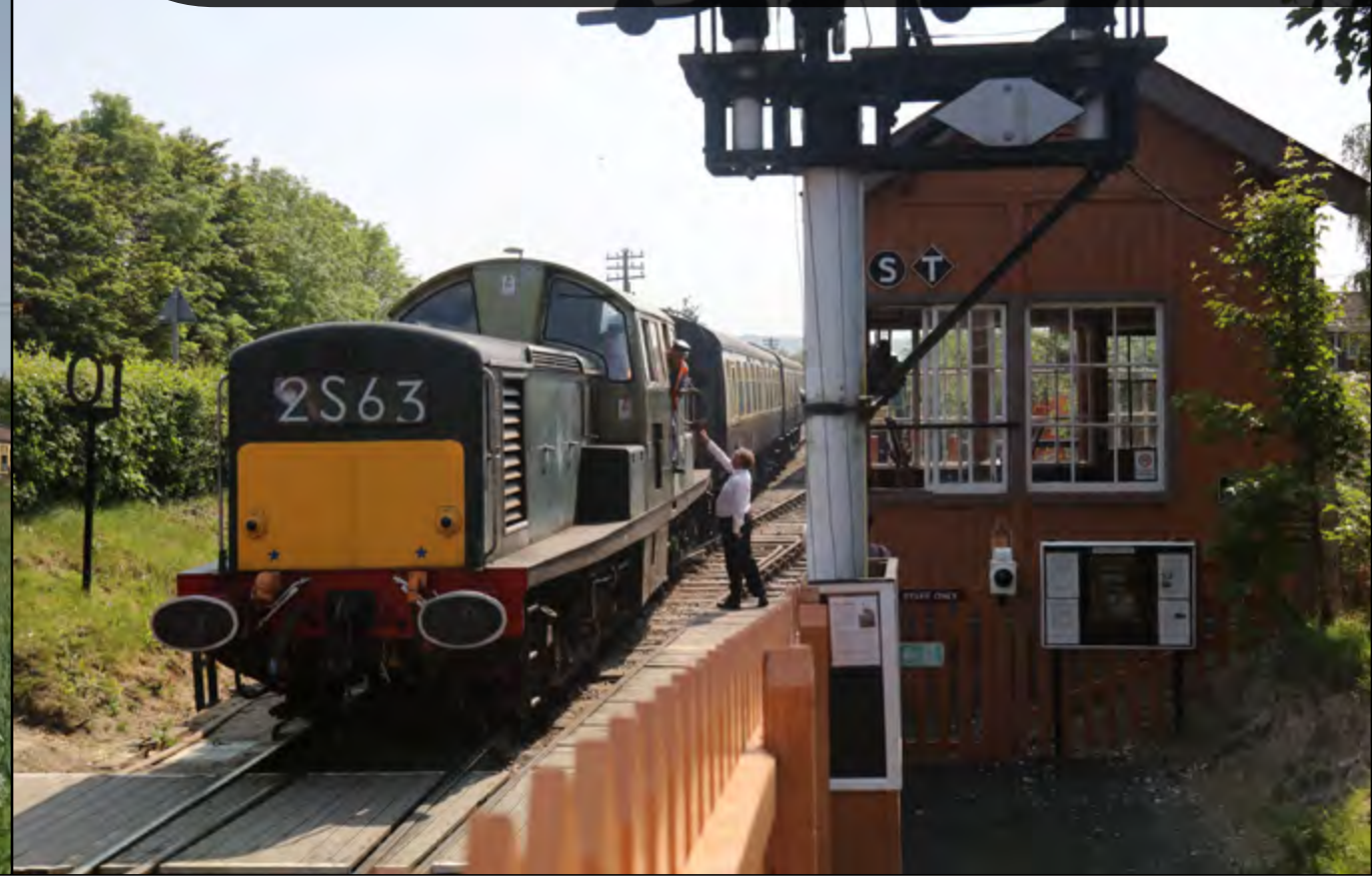
The signalman hands the token to the driver of sole surviving 'Clayton' No. D8568 as it brings in the stock for the 15:30 departure at Chinnor. Jeff Nicholls
