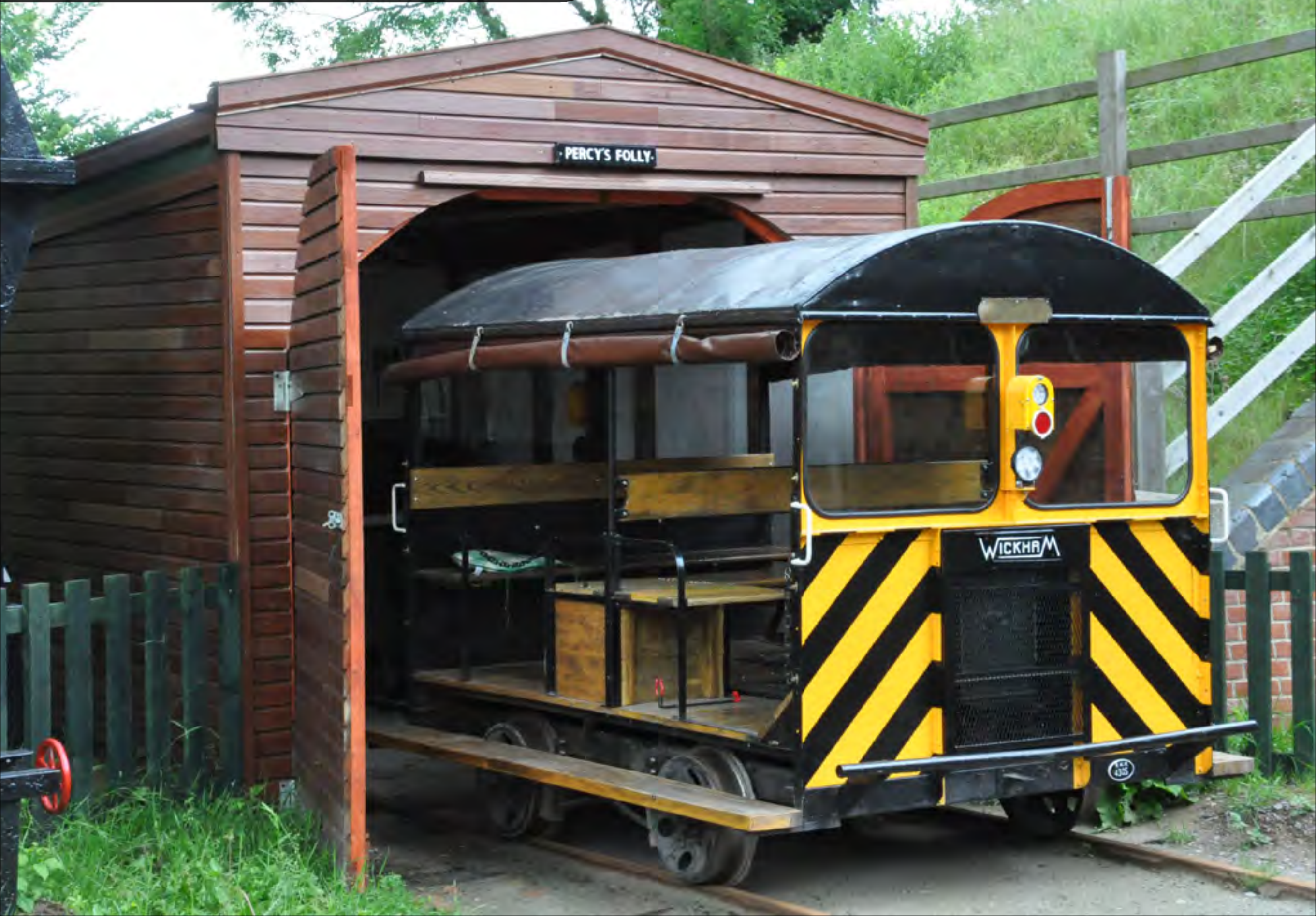
A preserved Wickham Type 27A Trolley is seen at Blunsden on June 22nd, housed inside its very own shed. Ken Mumford
