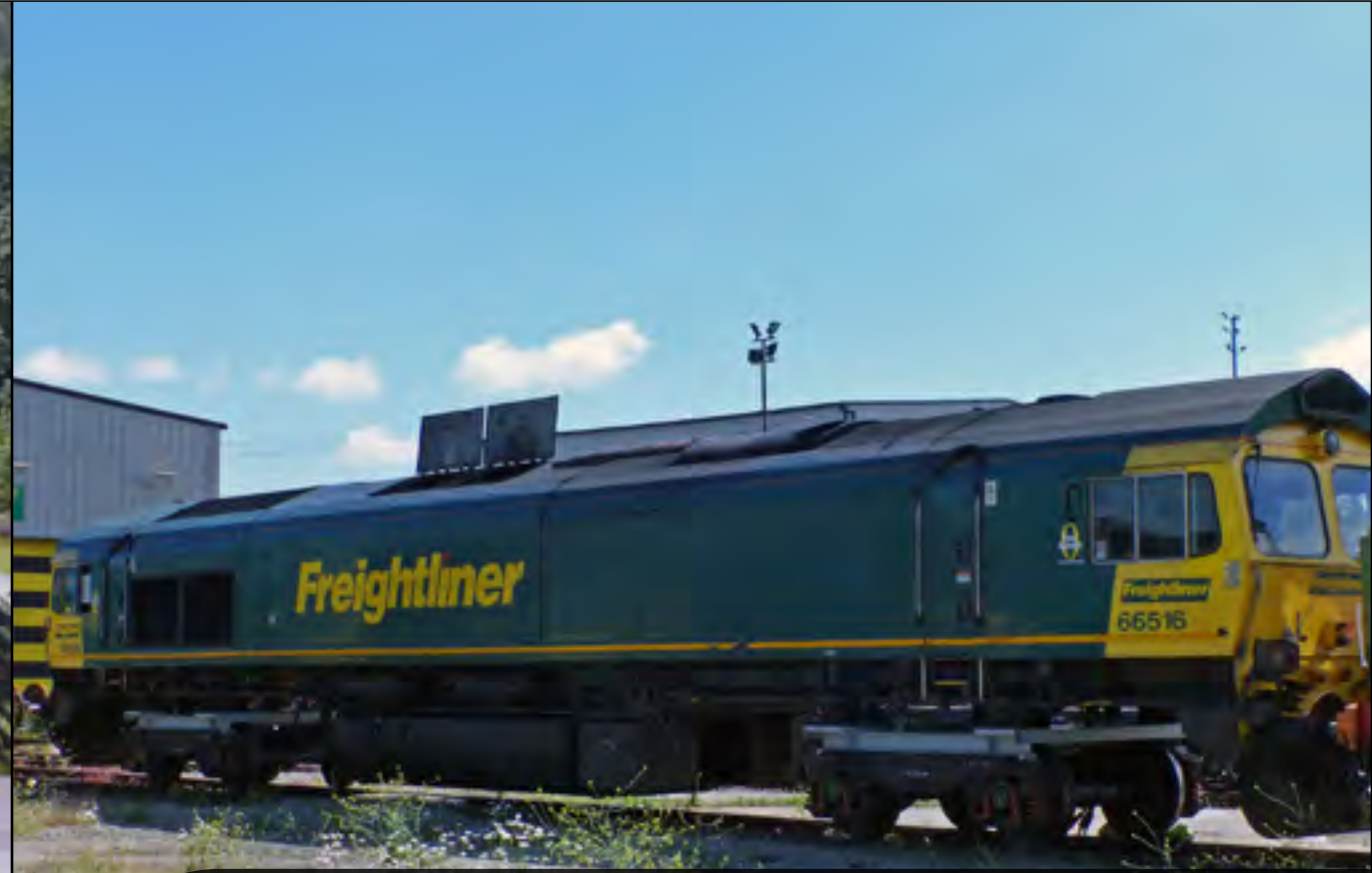
Class 66 516 is pictured undergoing maintenance at Leeds Midland Road on June 24th. Note the accommodation bogies. Michael Lynam
