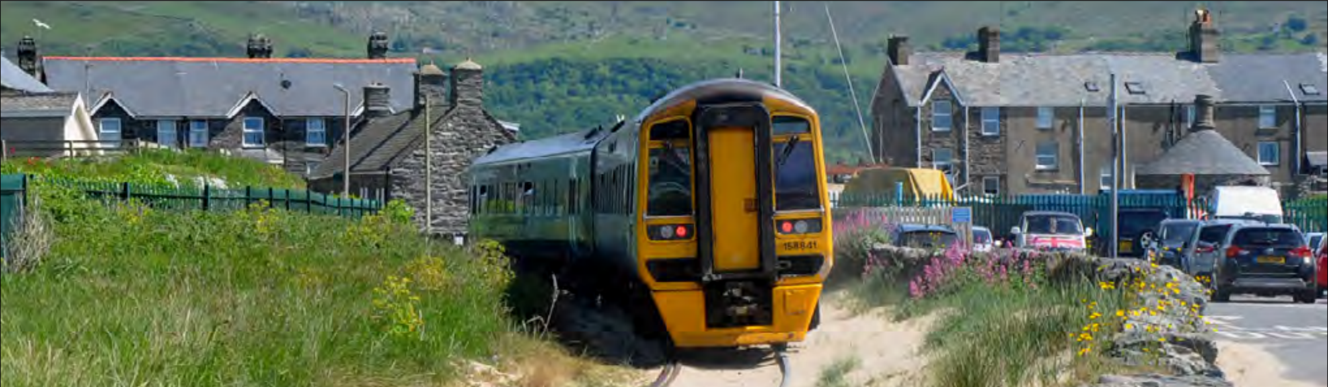
Though in many places the overgrown and sand-covered track was giving the impression of an abandoned railway, the Cambrian Coast Line in West Wales seemed to be well patronised by both locals and holidaymakers over the half-term holiday. All passenger trains are in the hands of the staple class of the line, the Class 158 DMU; only these units and a handful of converted Class 37 diesels have the correct ERTMS equipment to allow them to run on this test-bed line, which unfortunately precludes excursions, especially the once very popular steam-hauled summer trains of a few years back. Here Class 158 841 slowly pulls out of Barmouth and heads for the viaduct crossing the Afon Mawdach, with a train for Birmingham on June 1st. Ben Bucki
