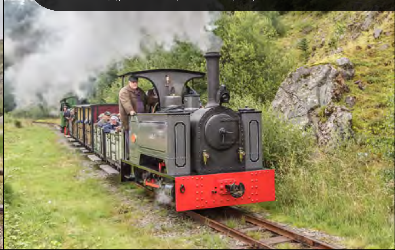
Newly restored and visiting from the Bala Lake Railway, Kerr Stuart 'Sirdar' Class 0-4-0T 'Diana' works No. 1158 of 1917 (with Bagnall 0-4-0ST 'Sir Tom' banking) attack the steep gradient as they head to the quarry face. Ken Abram
