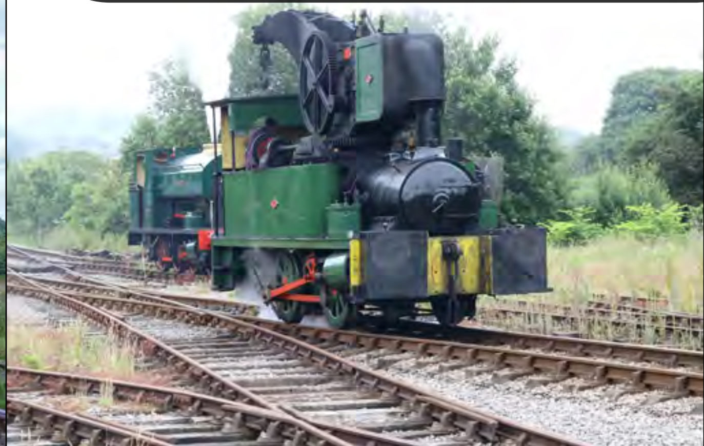
Always popular at the line is Dübs and Company crane tank 0-4-0T No. 4101 'Dubs', seen here at the colliery shunting mineral wagons. Class47
