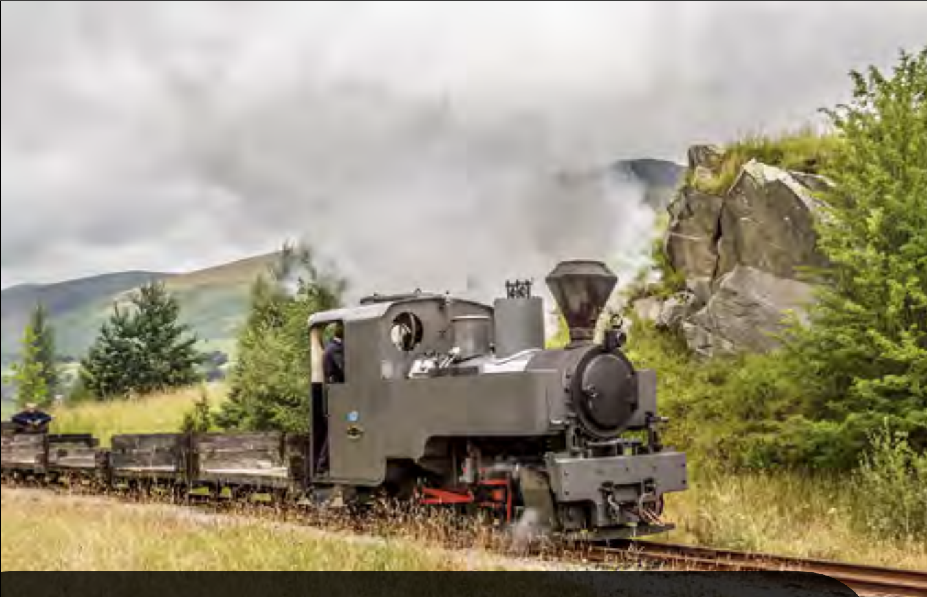
Kerr Stuart 'Joffre' Class 0-6-0WTT works No. 3014 of 1916 heads up the hill with some flat wagons to the head of the quarry. The loco was visiting from the Moseley Railway Trust's Apedale Railway. Ken Abram
