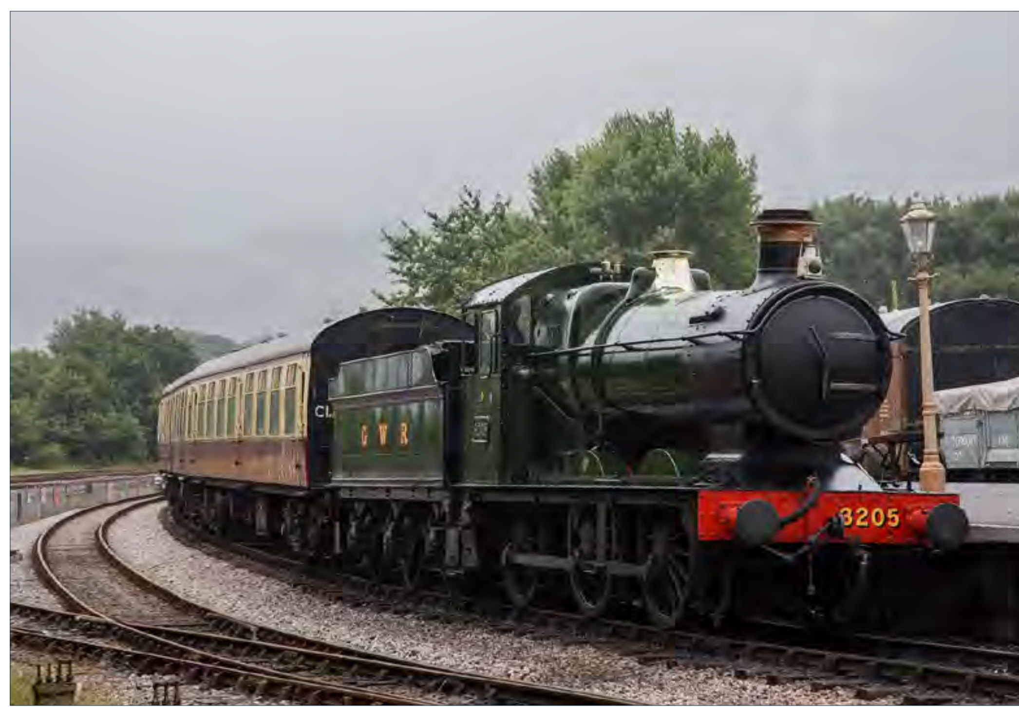
▶ GWR 0-6-0 No. 3205, built by the GWR in Swindon in 1946 and is the sole surviving member of the 120-strong 2251 Class of locomotives designed by C. B. Collett. Pictured here awaiting departure time from Totnes. Richard Hargreaves
