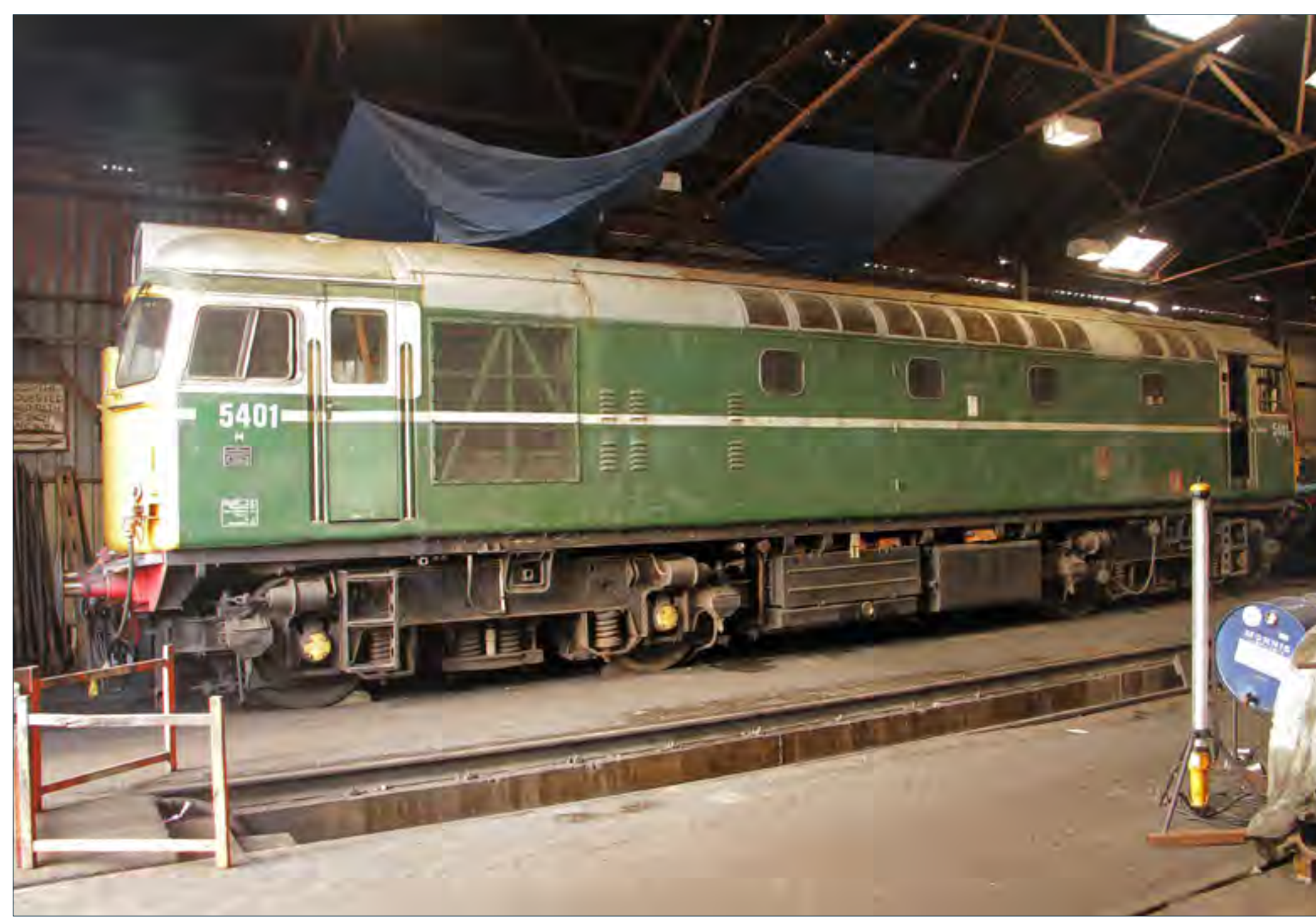
▶ BRCW Class 27 No. D5401 is seen undergoing repairs to the corroded cab window area at Loughborough. Derek Elston
