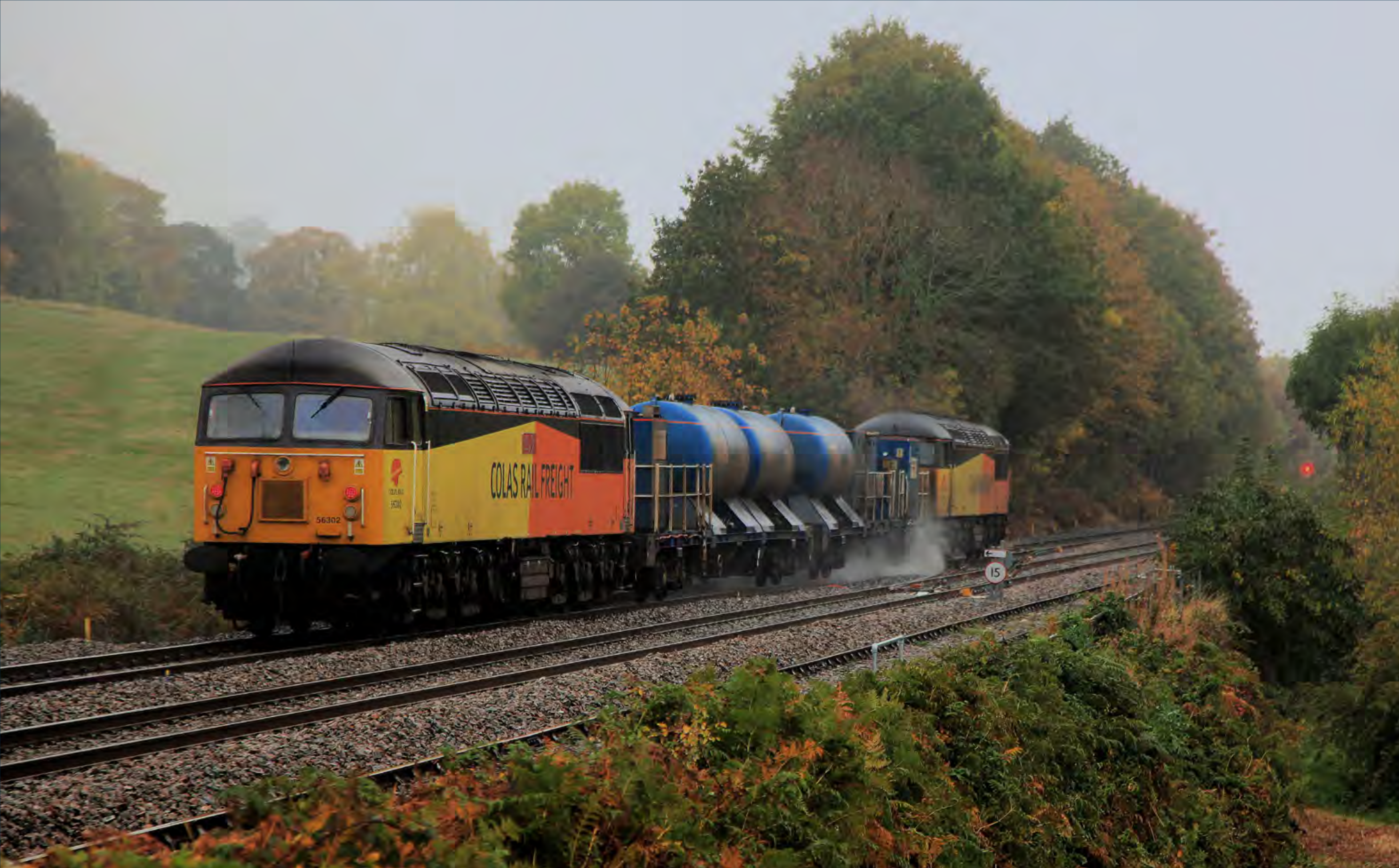
Colas Rail's Class 56 302 crosses Malvern Common at the rear of a rail head treatment train on October 29th. Neil Pugh
