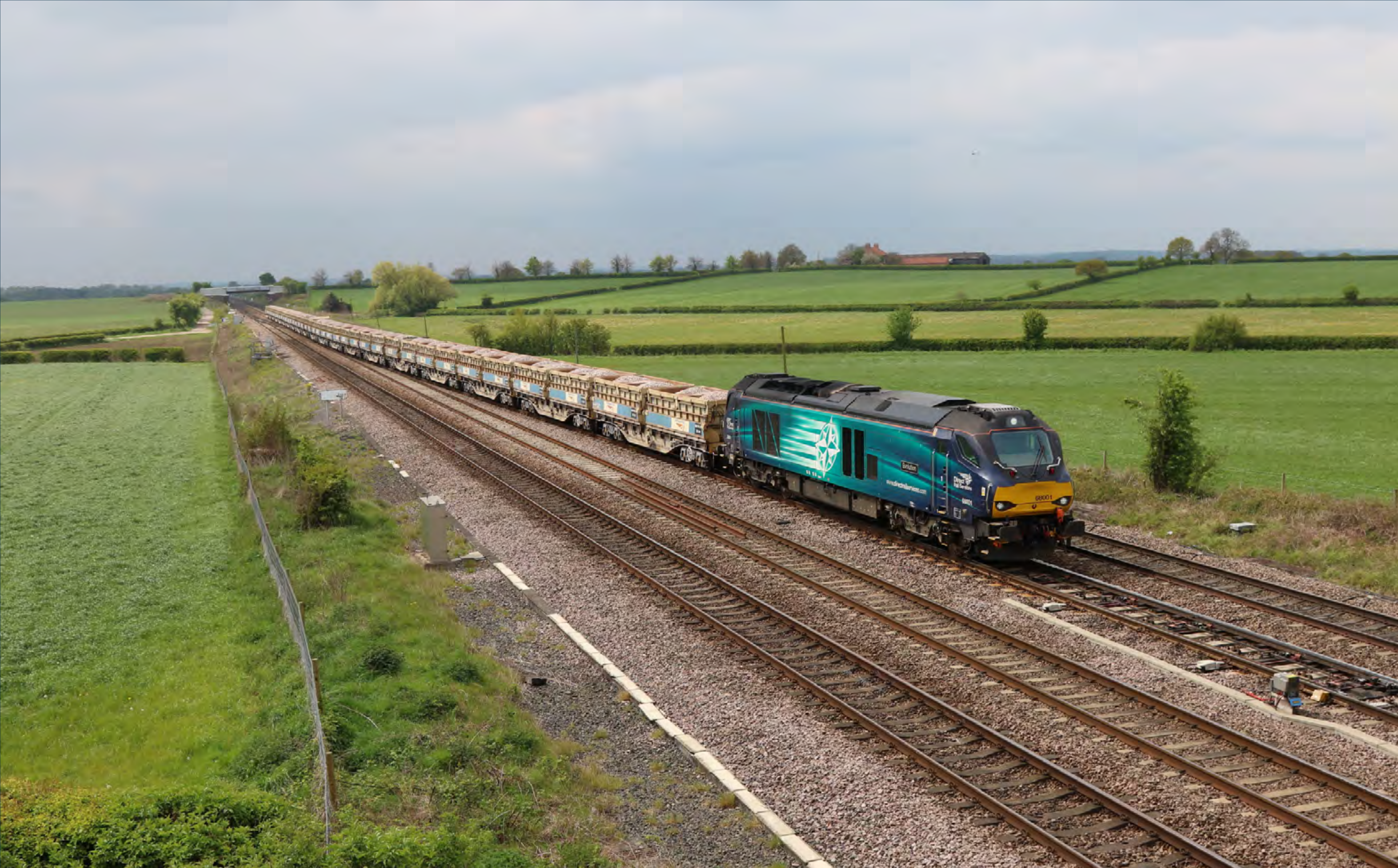
On May 2nd, Class 68 001 working a Mountsorrel - Carlisle Kingmoor loaded ballast, heads through Colton Jct. Alan Rigby
