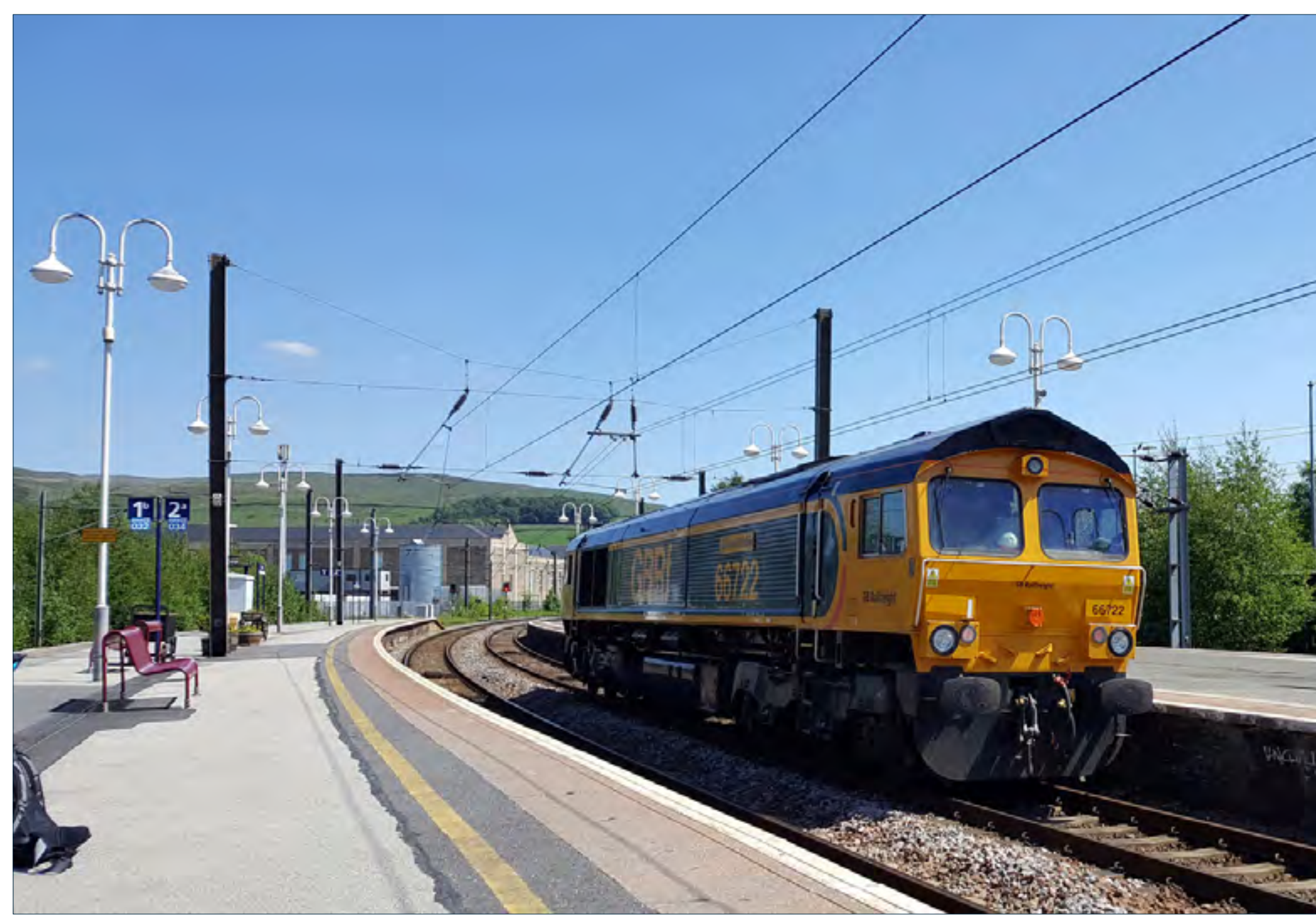
On May 31st, at Skipton, North Yorkshire, GBRf Class 66 722 'Sir Edward Watkin' crawls light engine through the station. The loco had arrived with train 6D72, empty wagons for the quarry at Grassington (reached via a reversal in the sidings outside the station) and the loco was using the platform roads to run-round. Ben Bucki
