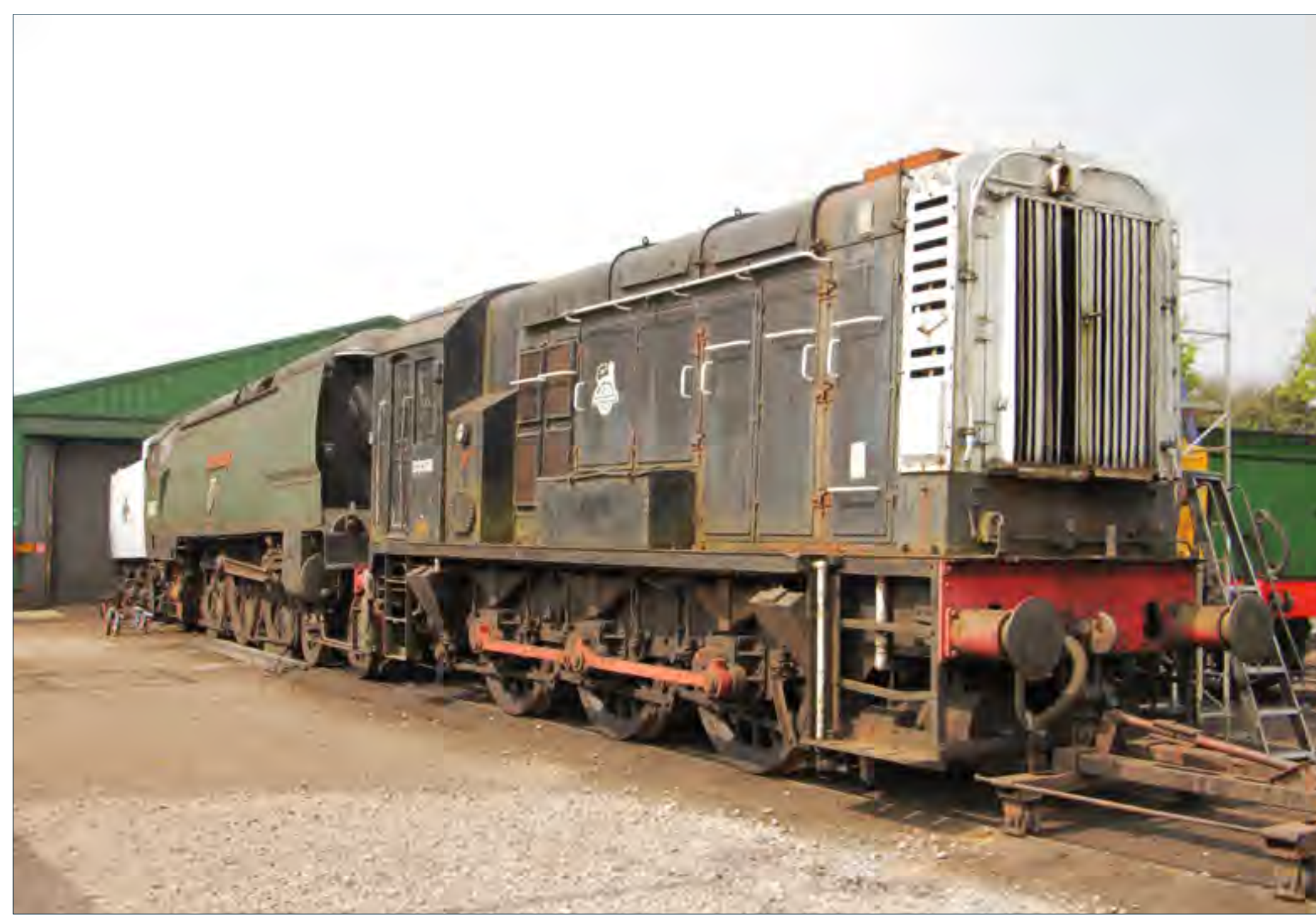
▶ A tatty looking English Electric 350hp shunter, No. D3358 stands on shed at Ropley on May 6th. Behind it is West Country Pacific No. 34007 'Wadebridge'. Derek Elston
