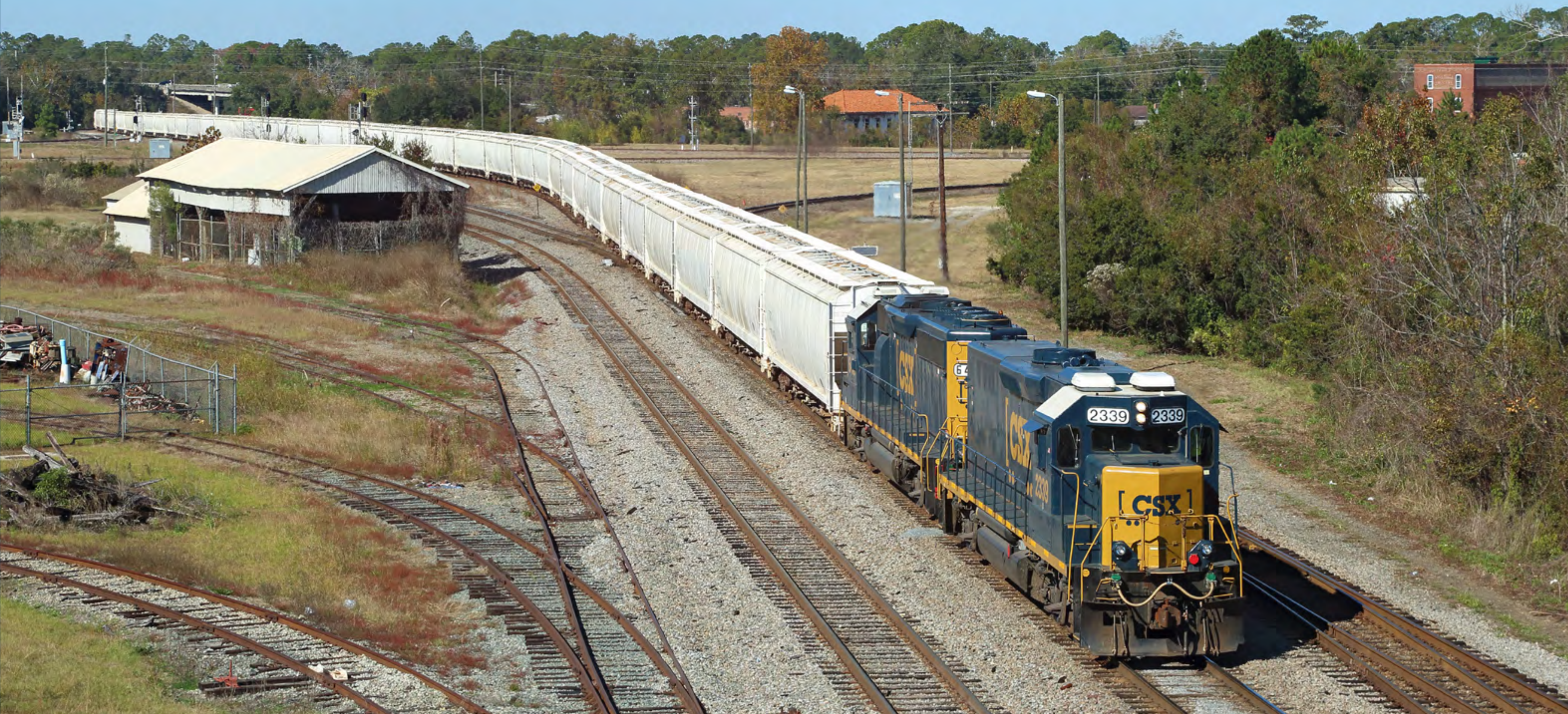
CSX Nos. 2339 (EMD Road Slug) and 6455 (GP40-2) cross the interlocking at Waycross. Laurence Sly
