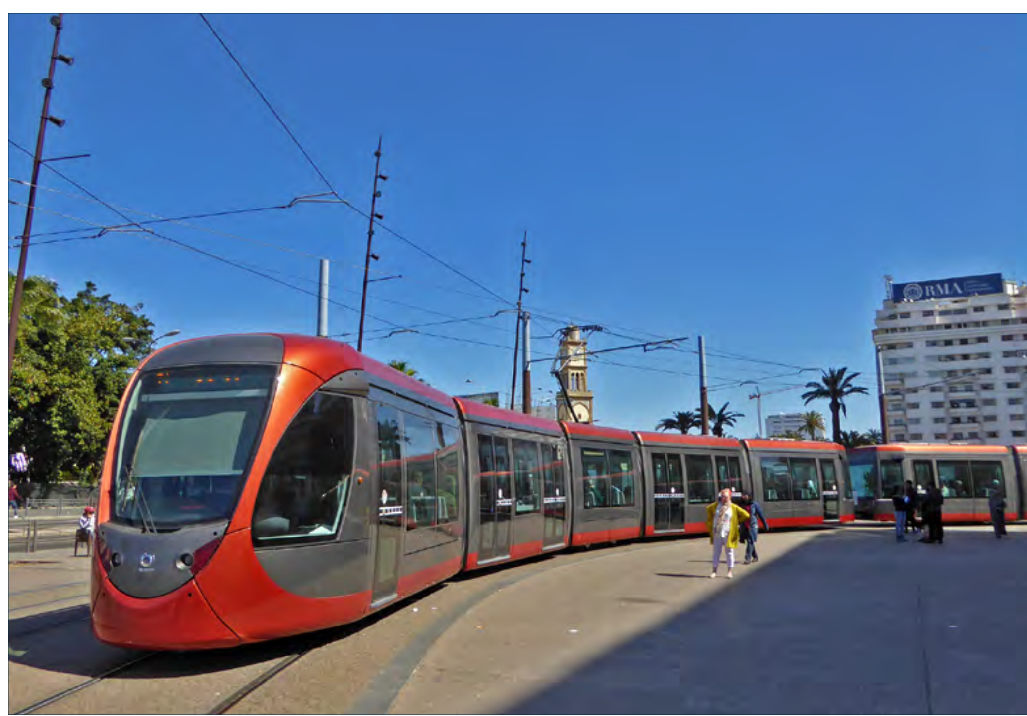
On March 30th in Casablanca, several Casa Trams are seen operating. The Casa Trams (RATP Group) operate a 31km line, using Alstom - Citadis type 302 low floor trams built by Alstom France. No fleet numbers are visible on the outside of the trams. Michael Lynam
