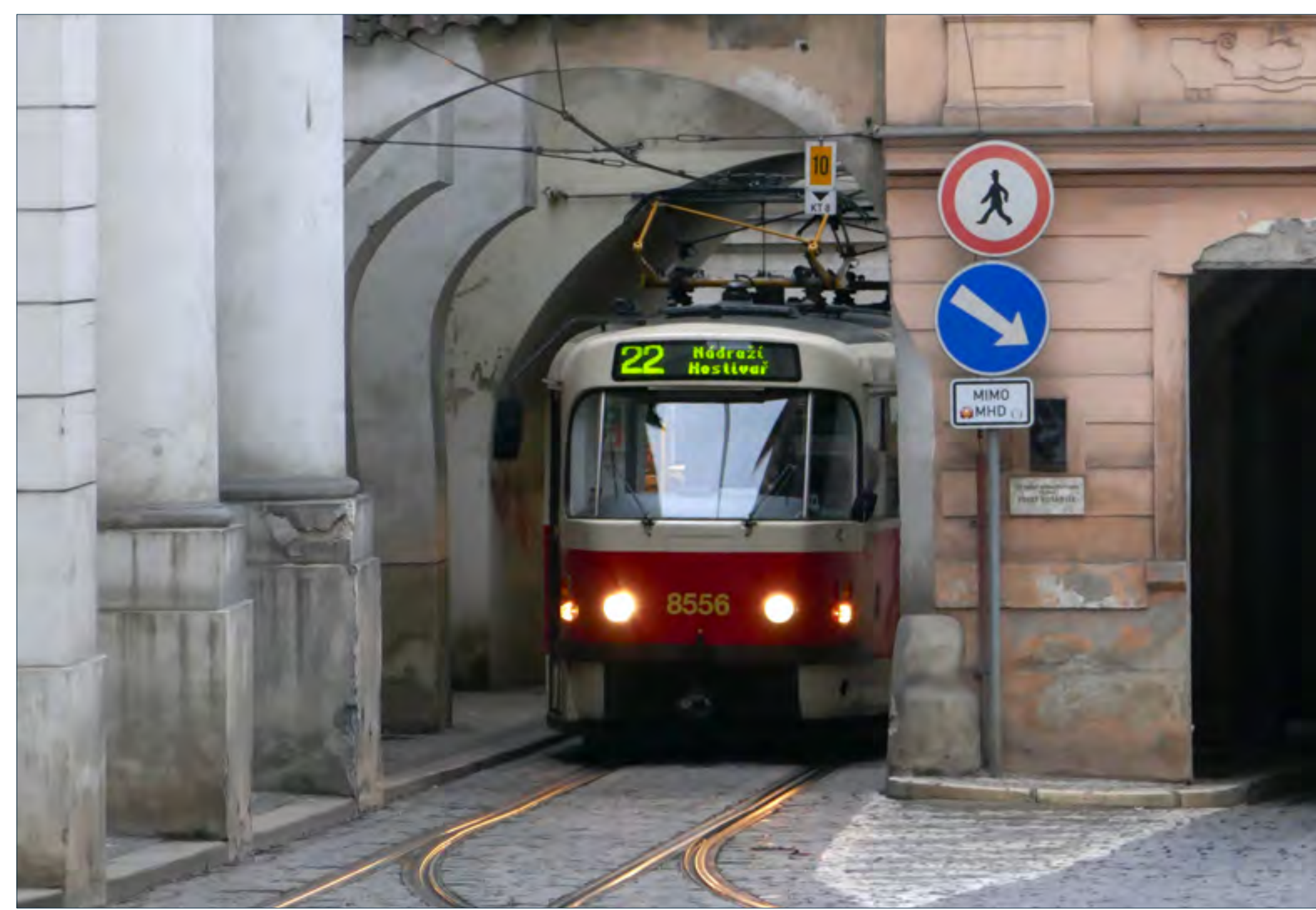
Prague Tatra built tram No. 8556 on the interlaced track threading the archway approaching the stop at Malostranské náměstí. Stearnsounds
