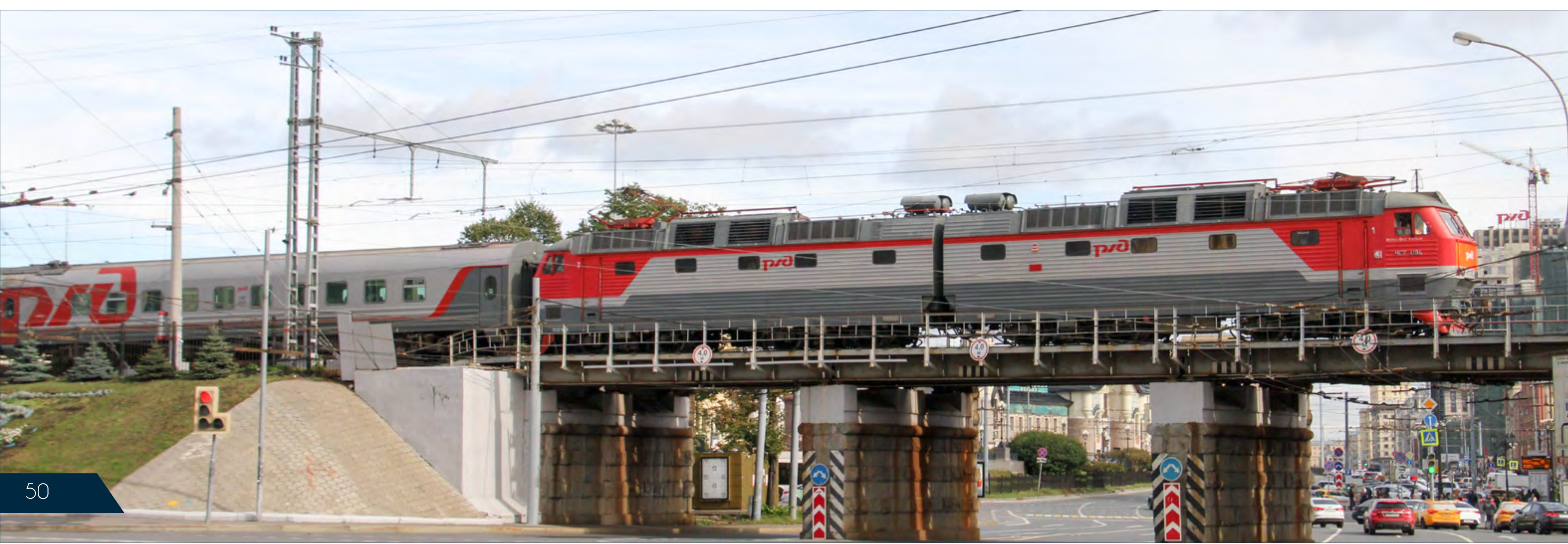
▶ Skoda built Class ChS7 consists of two sections and was produced between 1983 to 1999 at their V.I. Lenin plant in Plzen, Czech Republic. Here No. ChS7-084 passes Komsomolskaya Square in Moscow. Mark Enderby
