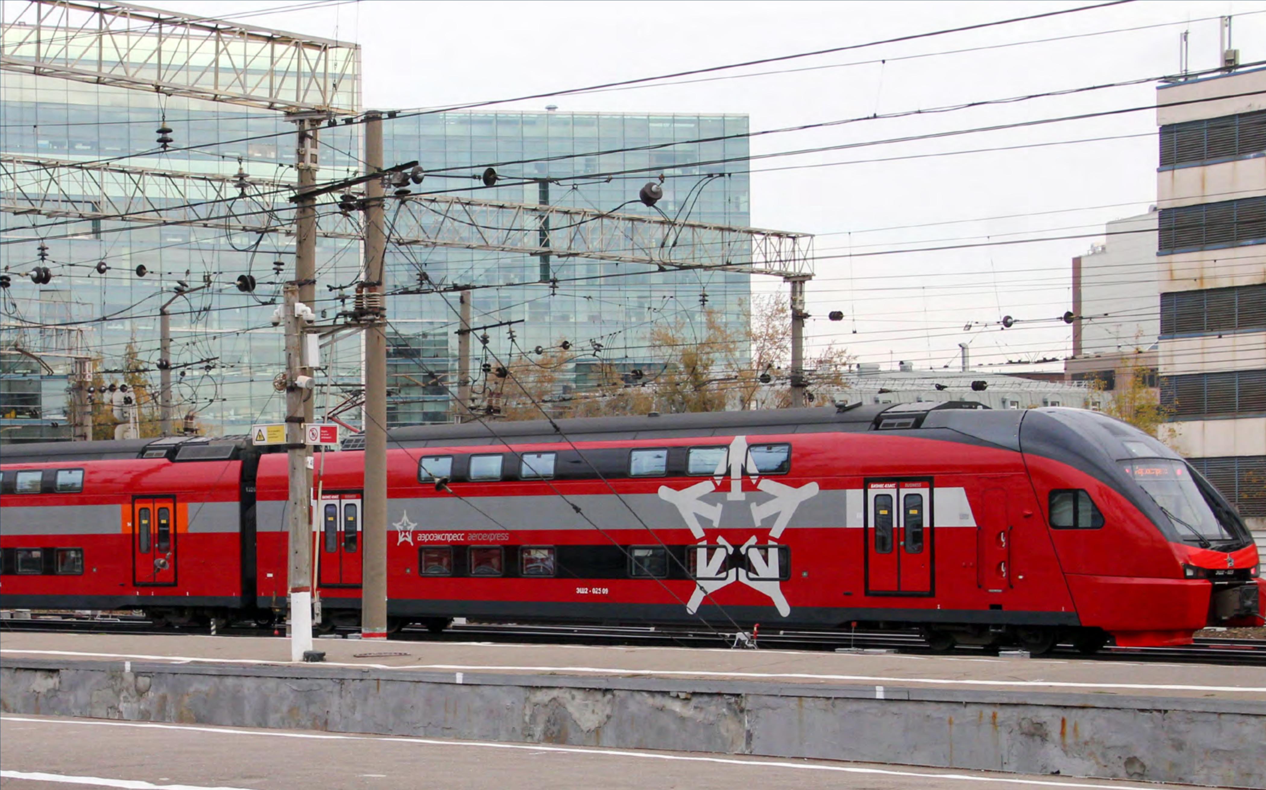
▶ The ESh2 'Eurasia' is the Russian gauge version of the 'Stadler KISS' double-deck EMU, seen here departing Moscow Paveletski with an 'Aeroexpress' service. Mark Enderby
