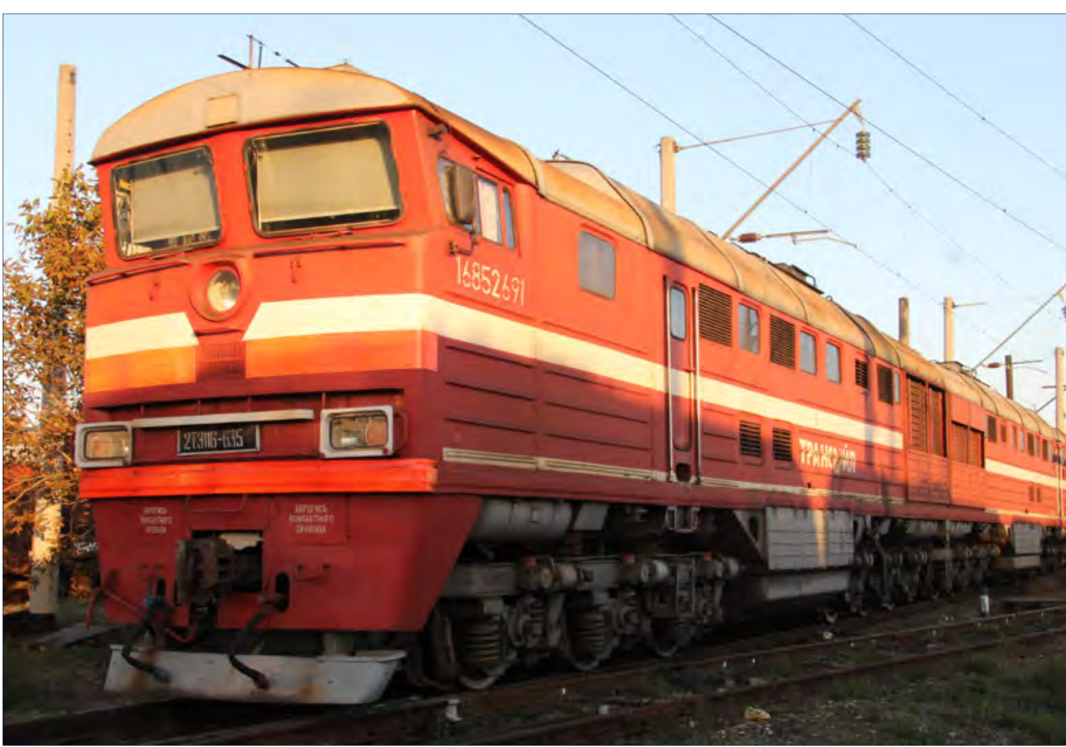
The 2TE116 is a broad gauge double diesel locomotive manufactured by Luhanskteplovoz, used extensively to haul heavy freight trains in the Soviet Union and its successor states, particularly by RŽD. No. 2TE116-635 is seen at Tikhoretsk depot. Mark Enderby
