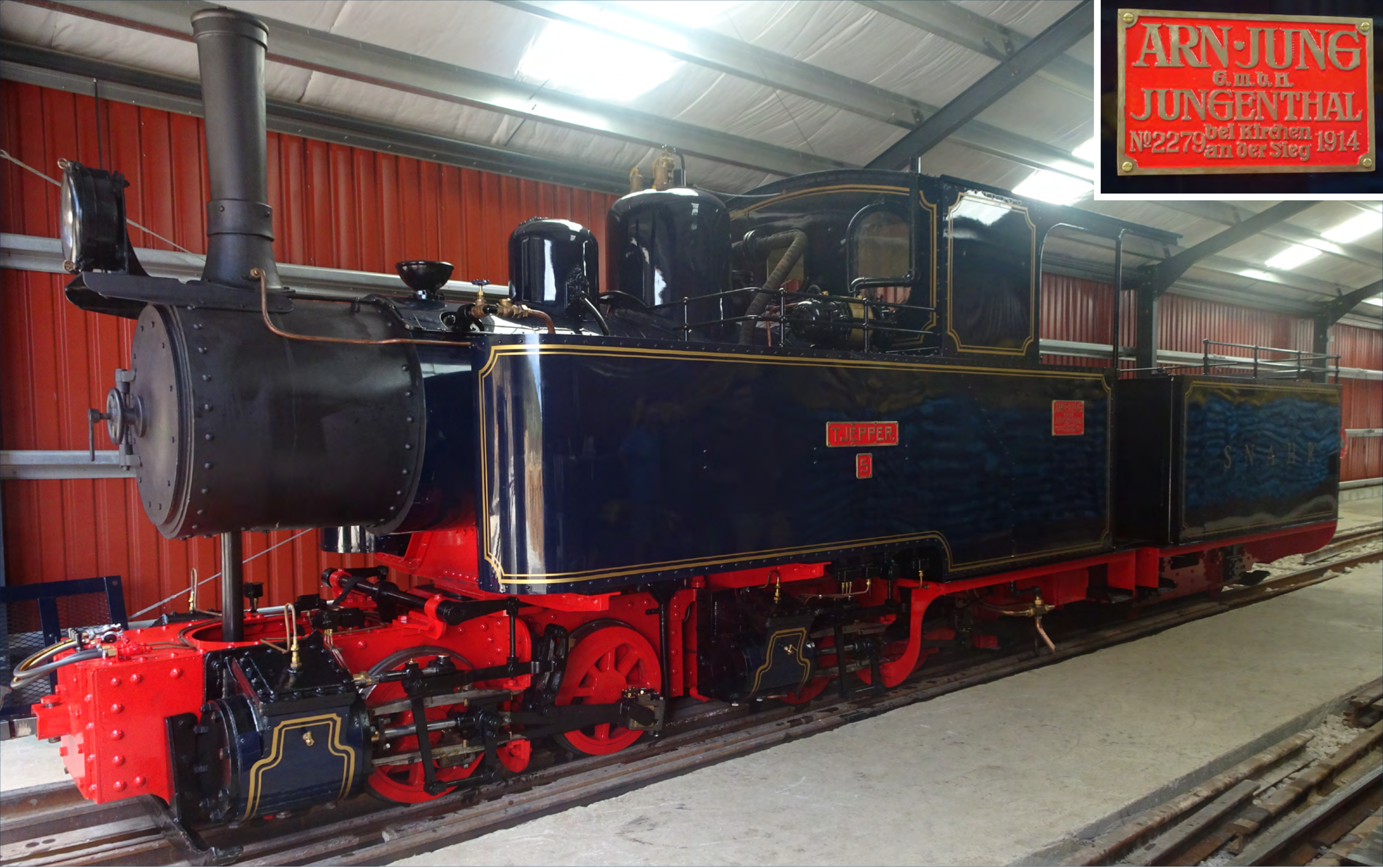
Photographed on February 11th, from inside the engine shed, just four days after delivery from Dover, England, to Saint Nicholas Abbey Heritage Railway, Cherry Tree Hill, St Peter, Barbados, West Indies. 0-4-4-0T 'Tjepper 5' was built in 1914 by Arnold Jung Lokomotivfabrik (Germany), works No. 2279. The gauge is 750mm (2ft 5 1/2") and it is an articulated locomotive of the 'Mallet' design with four Steam Cylinders driving 8 wheels. Its previous operator was the Ceper Baru Sugar Works, Java, but this engine has undergone redesign of specifications by Statfold Barn Railway, Tamworth, Staffordshire. (Modifications include supply of a tender, with a compartment at rear containing batteries for the brakes, alteration to the chimney spark catcher and large headlight on the front.). Allison Twycross
