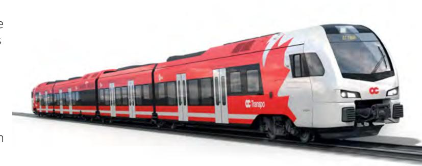
the current design the trains comply with the emission standard Tier4 final, with the North American Track Class IV, with ADA and are fully compliant with AODA (Accessibility for Ontarians with Disabilities Act) standards as well as with the North American fire safety standard NFPA 130.
