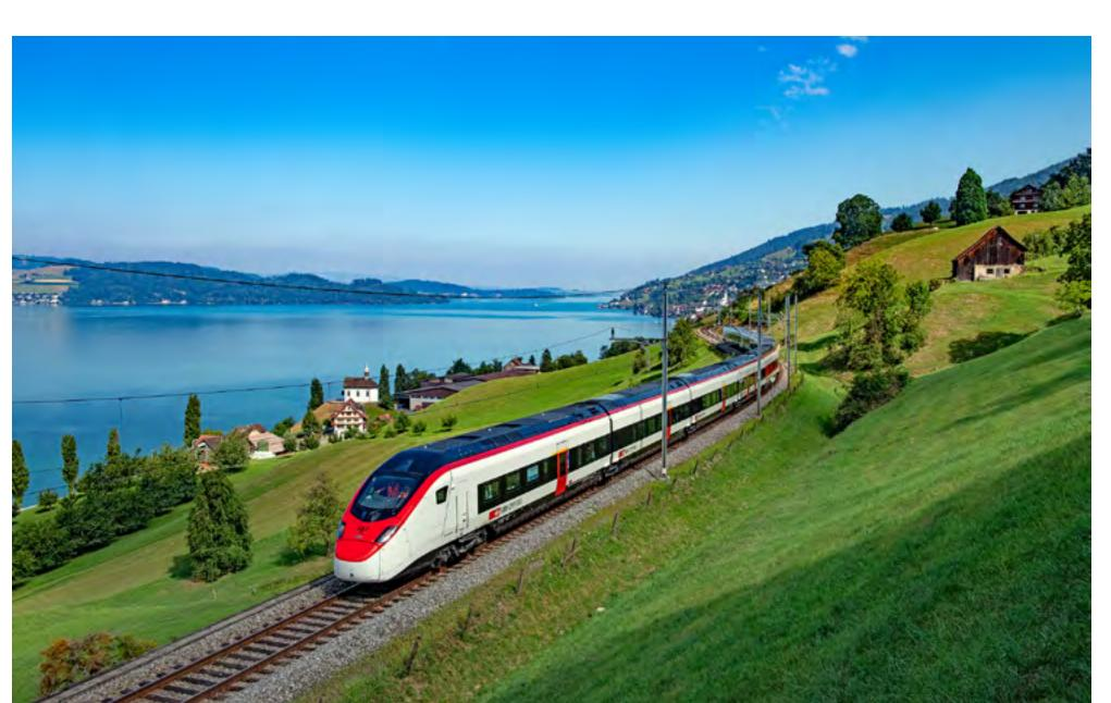
at speeds of up to 250 km/h. The vehicles are eleven-part electric multi-system units. Stadler developed and built the new train in just 23 months from the order date in October 2014 – only three months later it has been commissioned. It was presented to the public for the first time at InnoTrans 2016. Stadler calls the high-speed train family «SMILE», while the SBB has given them the name «Giruno», derived from the Rhaeto-Romanic word for buzzard.
