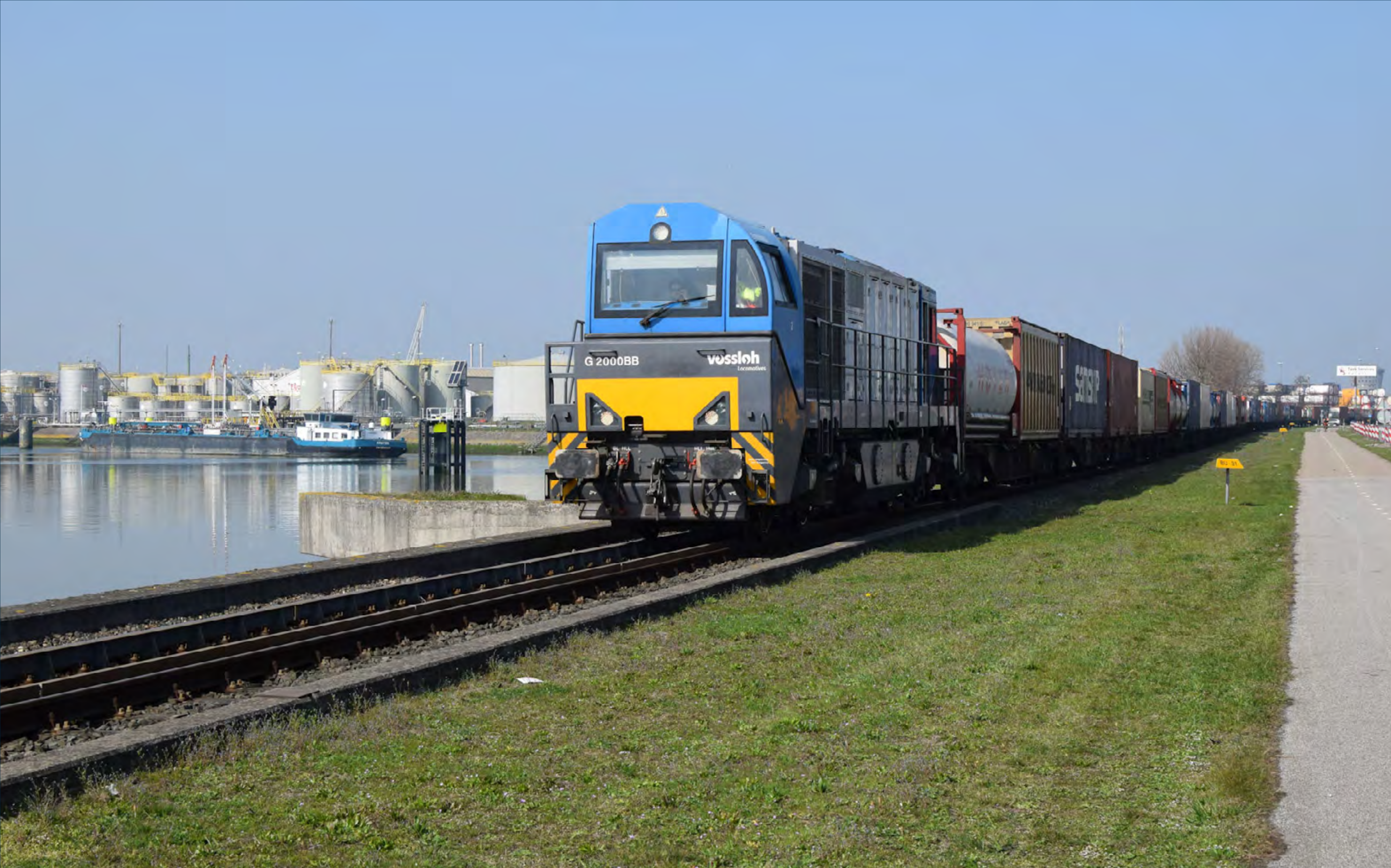
On March 29th, RTB Cargo Class G2000 (Vossloh, Kiel Germany) with an asymmetric cab pushes a container shuttle to the Combi Terminal Twente in Rotterdam. Erik de Zeeuw
