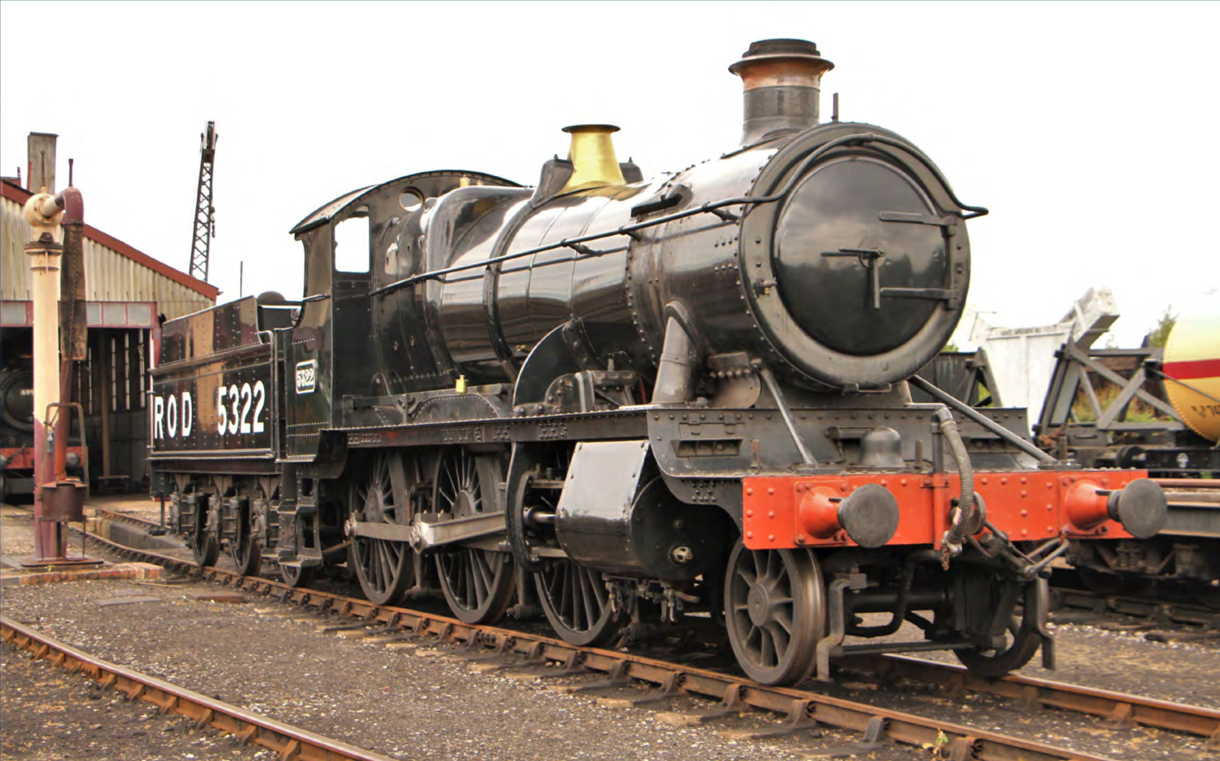
Churchward 43XX 2-6-0, 5322 stands outside the shed at GWS Didcot on June 2nd. Derek Elston
