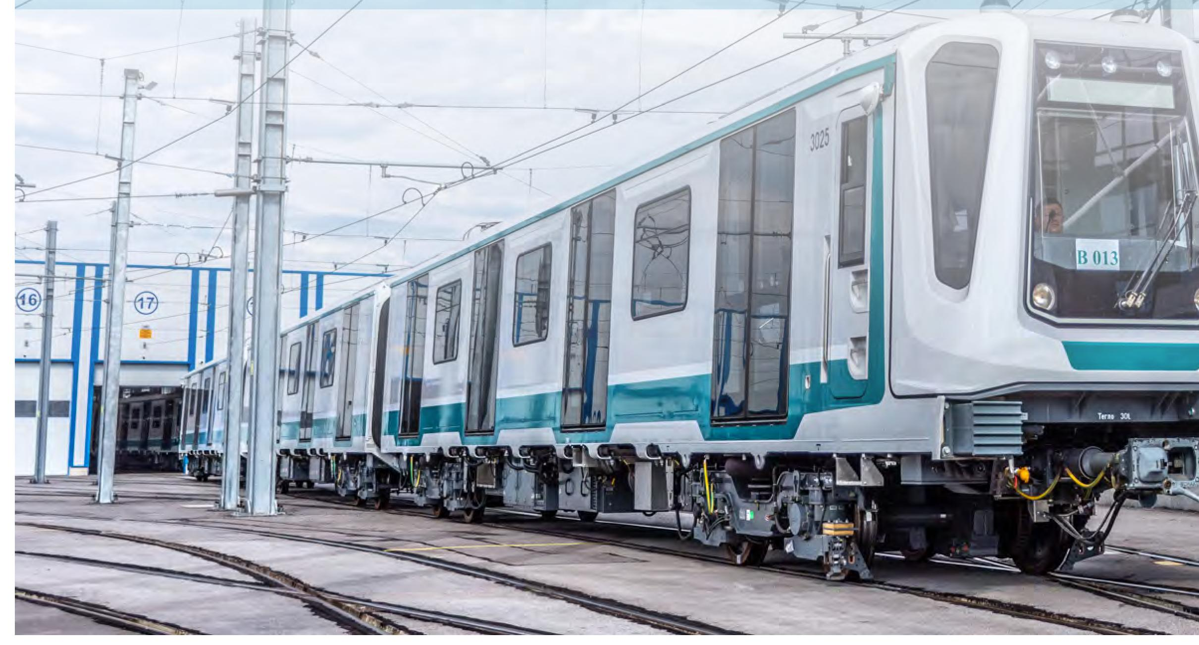
The trains can travel at speeds of up to 80 kilometres per hour. Their floor is a weight-saving, sound-absorbent composite cork-aluminum plate. They also feature a highly redundant traction and brake system (bogieoriented), ensuring a high level of availability and electrodynamic braking almost down to standstill.
