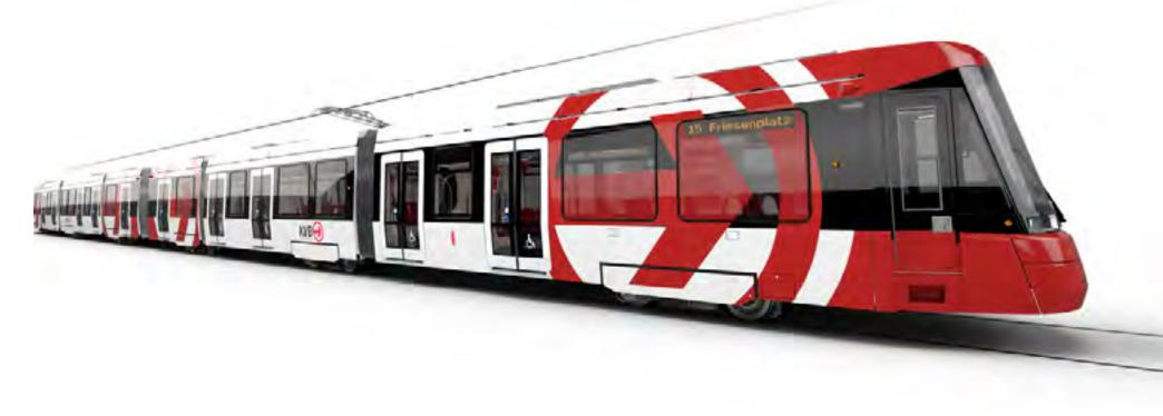
available, efficiently maintainable and includes a modern driver's workplace. As a contribution to traffic safety in the metropolis of Cologne, the new railways will be equipped with a collision warning system.
