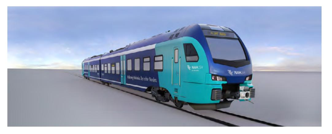
they're equipped with the corresponding batteries, the new, all-electric trains can even use routes without an overhead line. Northrail GmbH (Northrail), which belongs to the Paribus Group, will be supporting the project for the full duration, until 2052, which will initially entail intensive monitoring of the process for manufacturing the trains. Following successful delivery of the new trains, Northrail will also be in charge of the ongoing technical and business sides of asset management.
