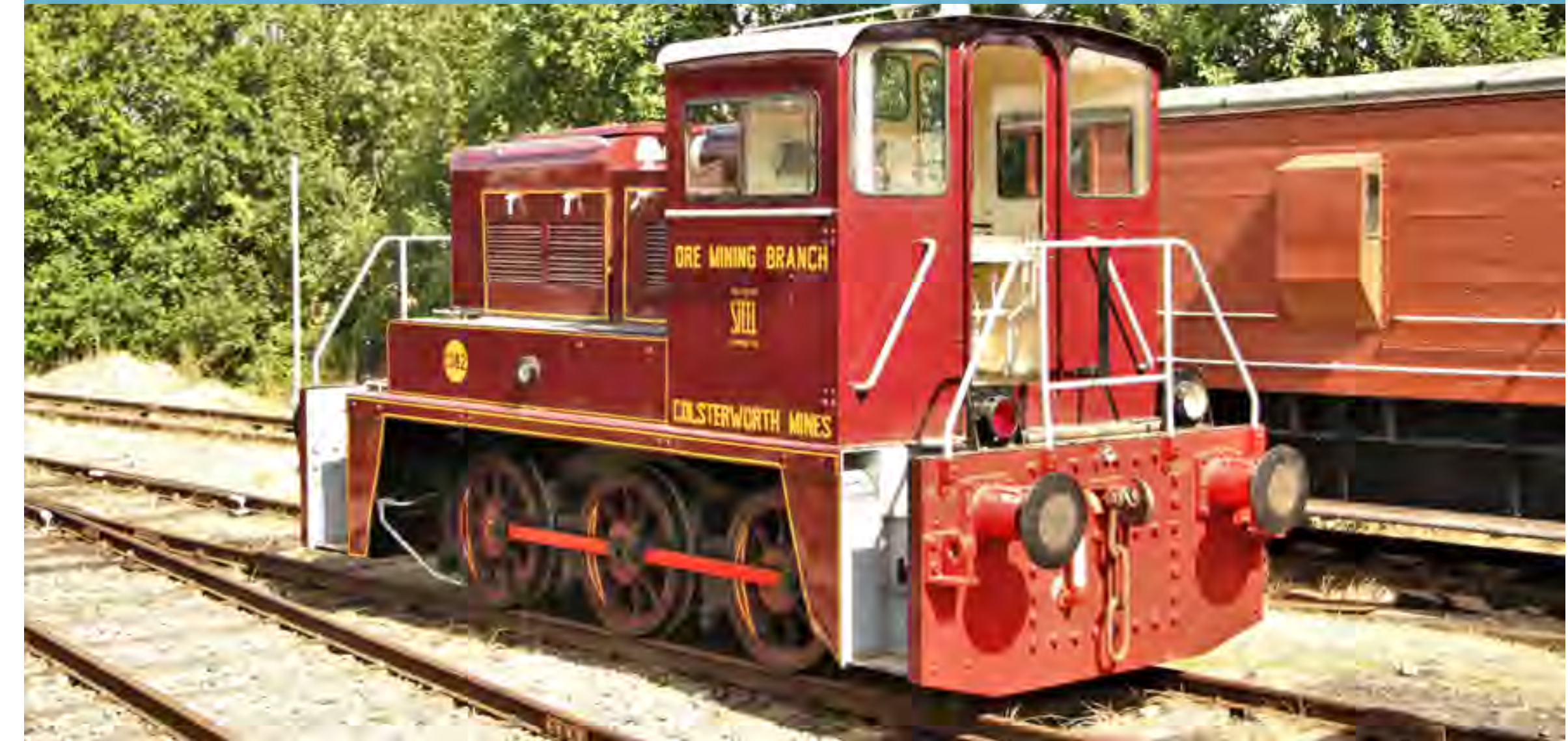
Yorkshire Engine Co. 0-6-0DE shunter, works No.2872, is seen in Colsterworth Mines livery at Rocks by Rail on August 15th. Derek Elston
