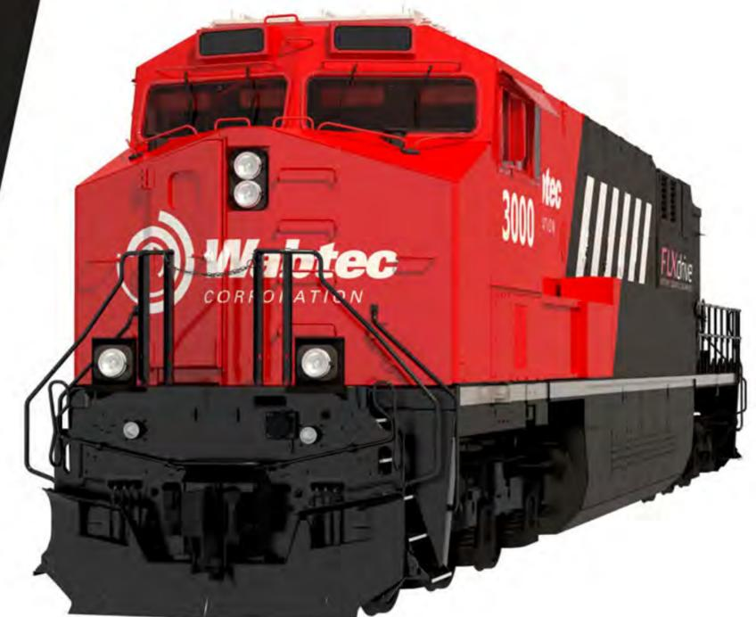
The FLXdrive battery locomotive is part of Wabtec's initiative to develop the next generation of zero-emission locomotives. The company has a clear path to power new locomotives – and repower existing locomotives – with batteries, hydrogen internal combustion engines, and hydrogen fuel cells.
