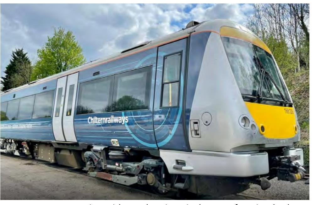
engine with an electric unit that can function both as a motor and as a generator. The battery system stores power that is recovered during train braking.
