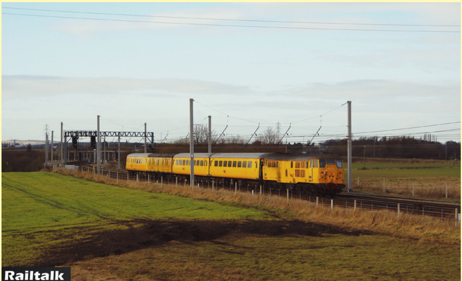
Above: Class 320 318 is seen calling at platform 1 of Dalmuir station working the 19.39 2E55 Springburn - Balloch service on the 17th March. Jonathan McGurk Below: Network Rail has been running some test trains using a single Class 31 and a DBSO in order to remove the need for a second Class 31. Here the Class 31, 31 105 was powering the train from the rear and the DBSO unit was driving the test train north through Winwick Jct on March 7th. Dave Harris
