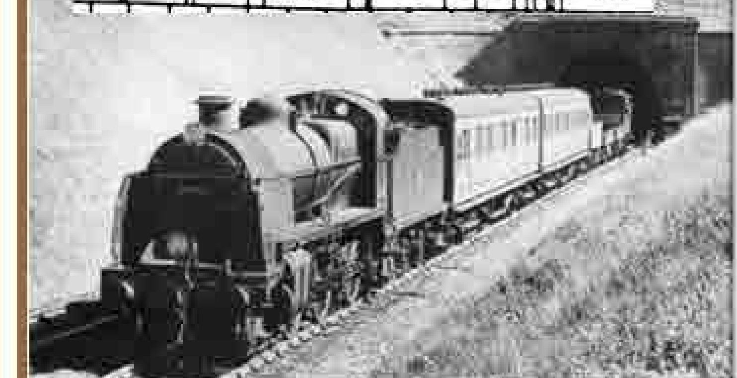
'N' class 2-6-0 No. 31835 leaves the west portal with a permanent way train which includes two elderly es-L.S.W.R. coaches.
