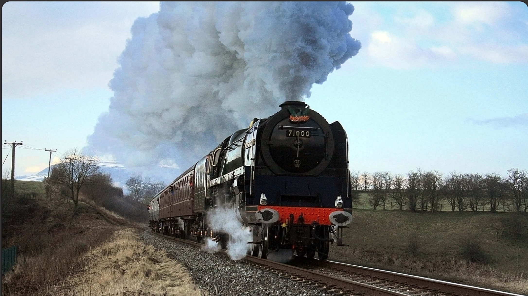
BR 8P No. 71000 "Duke Of Gloucester" powers through Burrs Country Park with a service from Rawtenstall to Heywood. The 8P is notorious for unreliability as it was originally an experimentally high powered locomotive produced by BR in the 1950s for express passenger trains, but the design failed to take off, and the Duke remained unique since the day she was built. On that weekend she had just returned to traffic following a long period in the works at Bury receiving an intermediate overhaul. Christopher Sutcliffe
