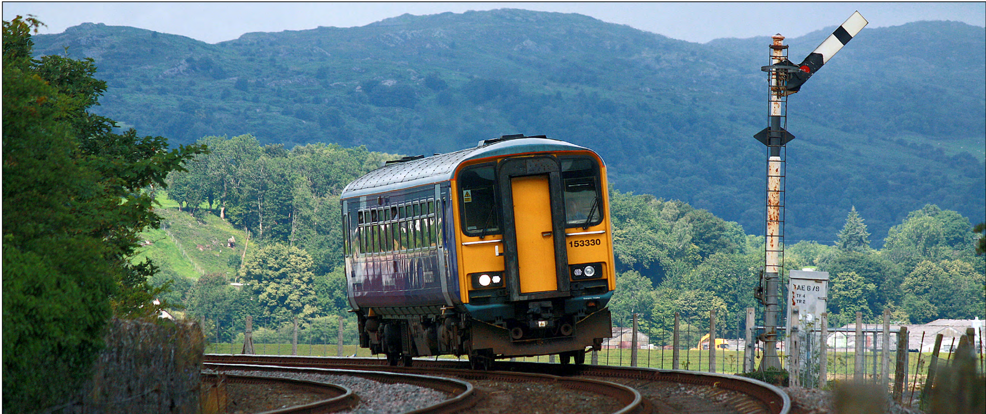
Above: Class 153 330 is working a Carlisle - Lancaster service southbound having just crossed Arnside viaduct approaching Arnside station. The line up at Arnside is still fully semaphore, and the box even retains it's original track circuit bells. CJ Sutcliffe Left: Class 66 100 is seen working a pipe train from Perth to Georgemas Jct. on August 31st. Richard Jones Right: Heathrow Express Class 332 009 has just arrived into London Paddington from Heathrow Airport on August 21st. Derek Elston
