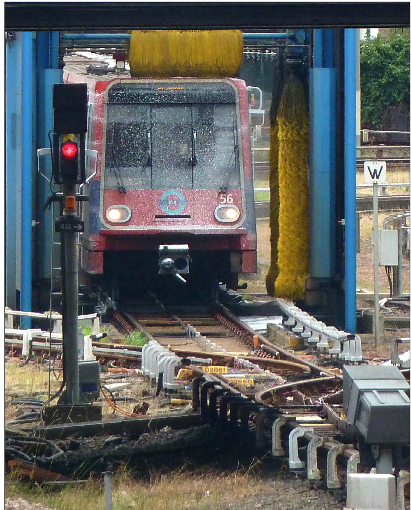
Time for a wash and brush up, as Docklands Light Railway No. 56 goes through the carriage washer at Poplar on August 18th. Andy
