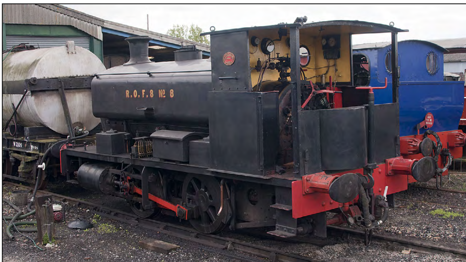
Below: Ex NCB 0-4-0ST No. 2157 built in 1943 by Andrew Barclay is currently undergoing restoration. Brian Battersby
