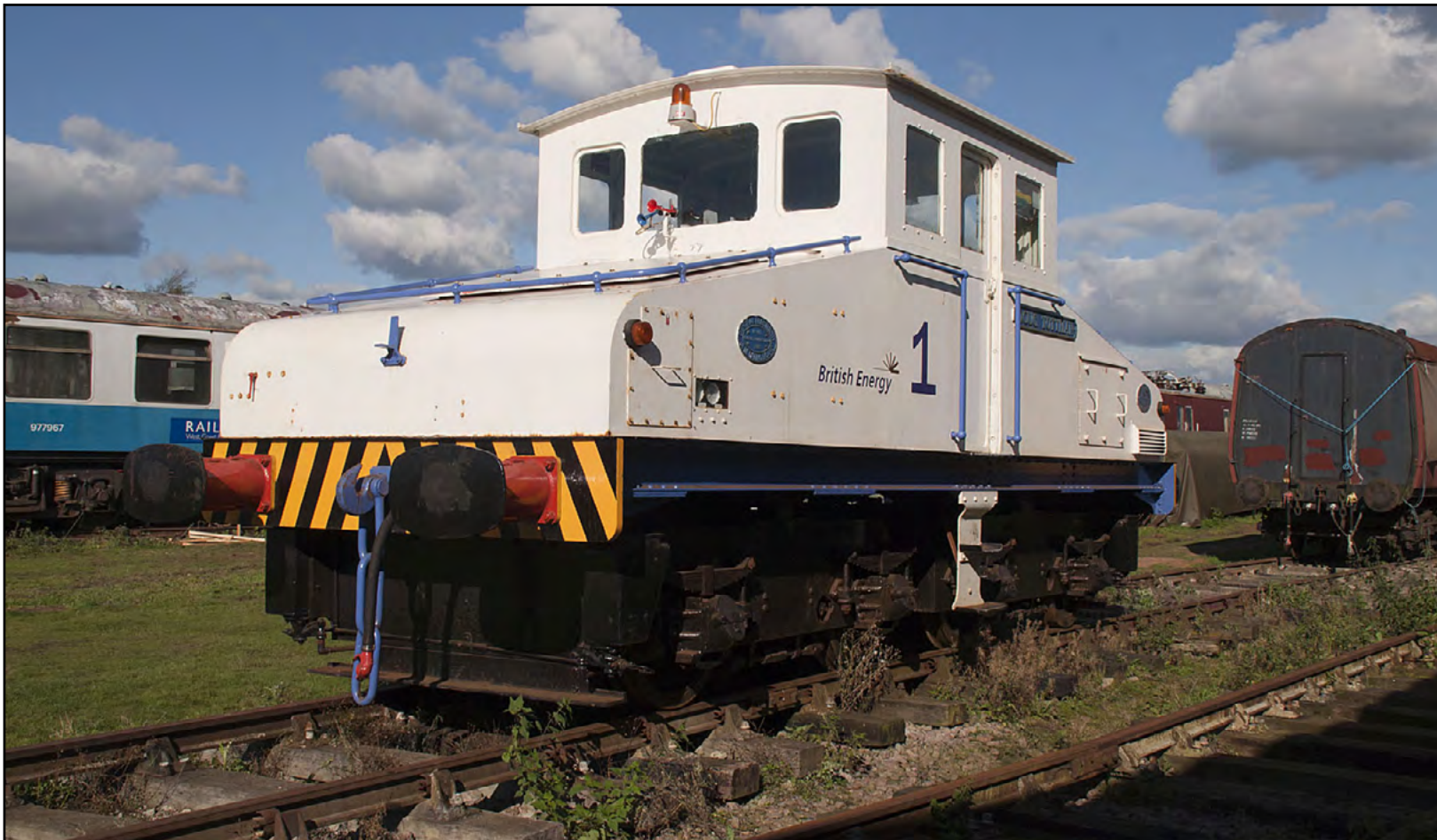
Below: One of several shunters at this fascinating location is Heysham Power Station No. 1, a Bo-Bo Battery Electric Loco built in 1945 by Robert Stephenson and Hawthorns. Brian Battersby
